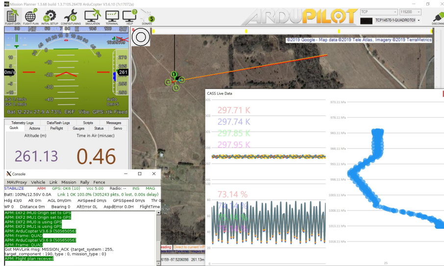
Figure 3. Screen capture of the simulator’s graphical user interface in which every flight parameter is displayed as if flying a real UAS. The UAS is represented by the green quadcopter in the map provided by Google (©2019 Google - Map data: ©2019 Tele Atlas, Imagery ©2019 TerraMetrics), the heads up display (HUD) in the top left corner shows the necessary avionics for the operator. The inset picture in the bottom right corner is a live view of the simulated temperature and humidity data interacting with the simulated UAS. Work is underway to better represent the vertical temperature and humidity profiles in the simulator.
