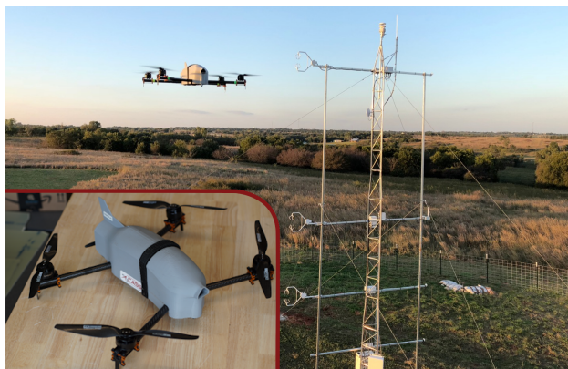
Figure 1. Picture of the CopterSonde UAS hovering next to a 10 m experimental flux tower. The picture in the bottom left corner shows a close up of the fully assembled CopterSonde UAS.
