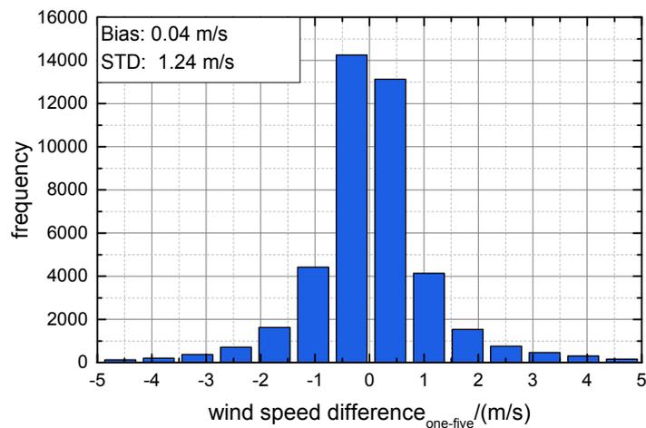
**Figure 3.** Histogram of the difference of wind speeds derived from 2- $\mu$ m DWL data by means of one scanner revolution and five scanner revolutions ( $v_{2\mu\text{m}_1\text{-scan}} - v_{2\mu\text{m}_5\text{-scans}}$ ) for all flights performed during the AVATARE campaign (see also table 1). The mean and the standard deviation (STD) of the data are indicated by the inset.
