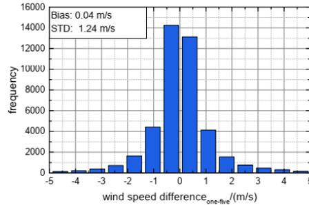
**Figure 3.** Histogram of the difference of wind speeds derived from 2- $\mu\text{m}$  DWL data by means of one scanner revolution and five scanner revolutions (one minus five) for all flights performed during the AVATARE campaign (see also table 1). The mean and the standard deviation (STD) of the data are indicated by the inset.
