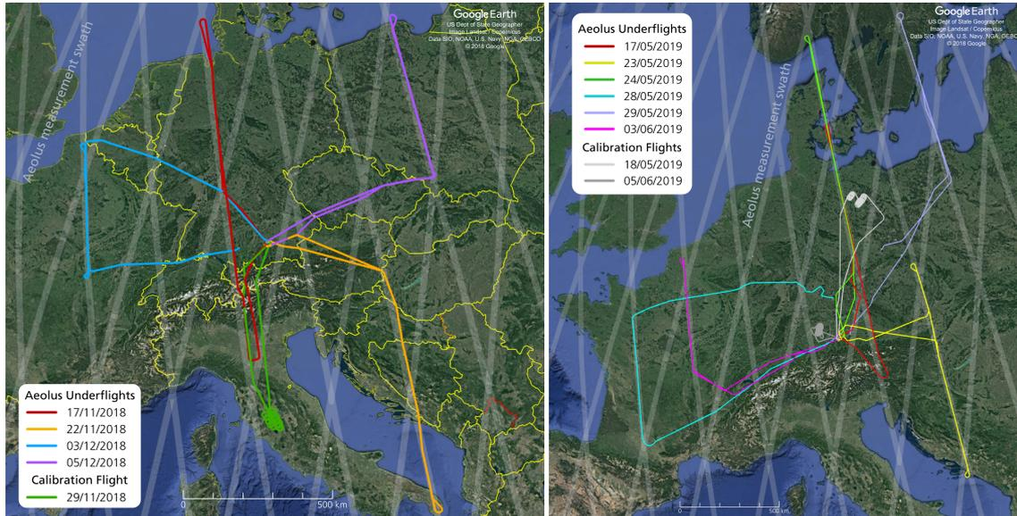
**Figure 1.** Flight tracks of the Falcon aircraft during the WindVal III campaign performed from 17 November 2018 to 5 December 2018 (left) and the AVATARE campaign performed from 17 May 2019 to 3 June 2019 (right). Each color represents a single flight. The Aeolus measurement swath is shown in gray color. During the probed evening satellite tracks, the Aeolus moving direction was always from south to north (ascending orbit).
