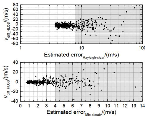
**Figure 6.** Wind speed difference of Aeolus HLOS winds and 2- $\mu\text{m}$  DWL winds projected onto Aeolus viewing direction according to Eq. (2) depending on the estimated error given in the L2B product for Rayleigh winds (top) and Mie winds (bottom). Shown are all valid data points from WindVal III and AVATARE. Data points with an estimated error larger than 8 m/s (Rayleigh) or rather 4 m/s (Mie) are not considered as valid observations (gray areas).
