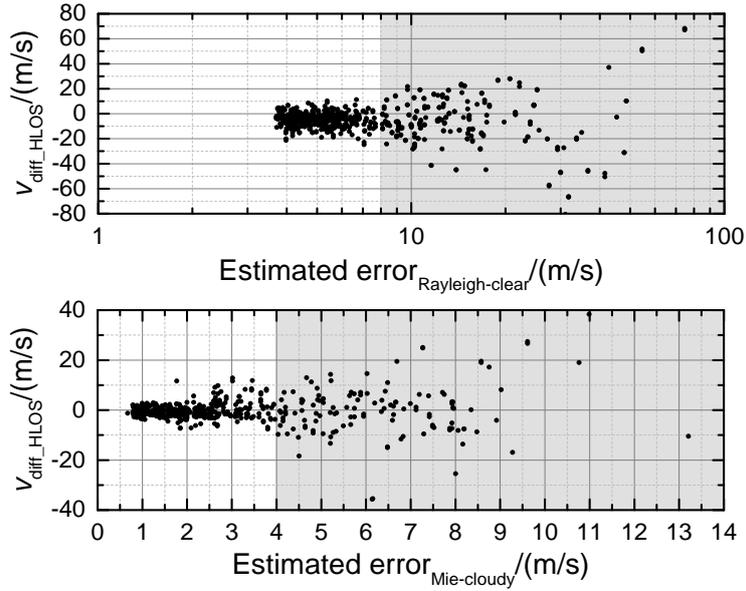
**Figure 6.** Wind speed difference of Aeolus HLOS winds and 2- $\mu$ m DWL winds projected onto Aeolus viewing direction according to Eq. (2) depending on the estimated error given in the L2B product for Rayleigh-clear winds (top) and Mie-cloudy winds (bottom). Shown are all valid data points from WindVal III and AVATARE. Data points with an estimated error larger than 8 m/s (Rayleigh) or rather 4 m/s (Mie) are not considered as valid observations (gray areas).
