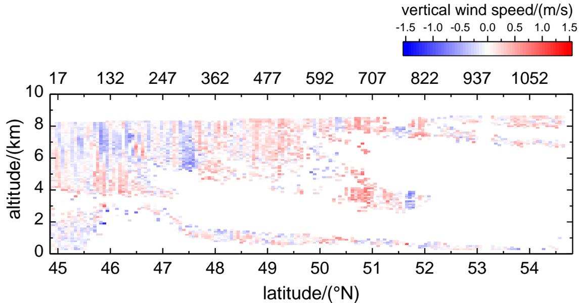
Figure 2. Vertical wind speed retrieved from 2- $\mu$ m DWL data by means of the MFAS algorithm for one scanner revolution during the first ever Aeolus underflight performed on 17 November 2018 during the WindVal III campaign (corresponding horizontal wind speed is shown in Figure 1). White colors indicate areas with no valid wind measurements due to aerosol-poor atmospheric conditions and a corresponding insufficient SNR.
