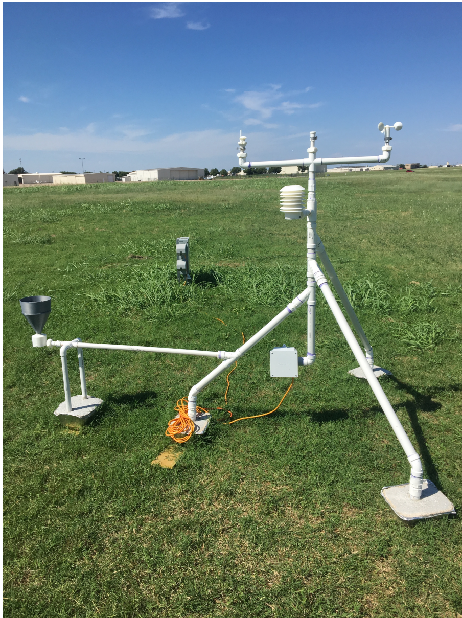
Figure 1. 3D-printed weather station initial installation in the field.
