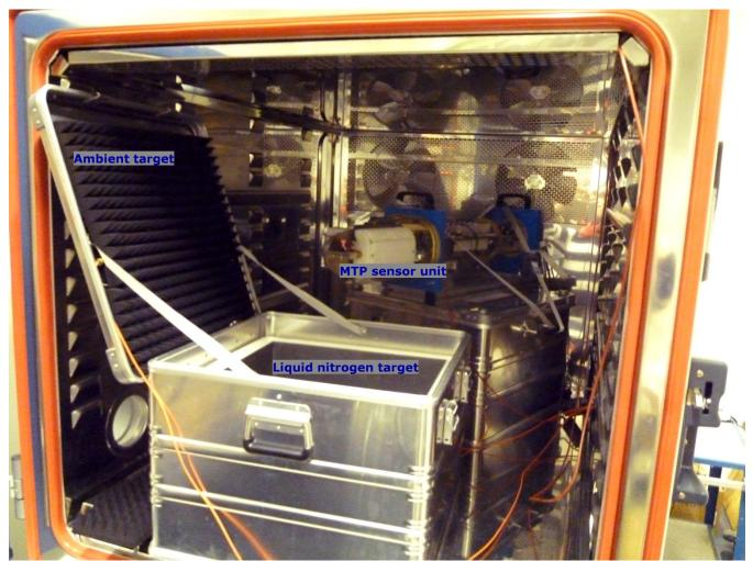
Figure 3: DLR-MTP inside the cold-chamber. For the measurements, the box containing the liquid nitrogen and the ambient target was rotated to face towards the MTP sensor unit. A second microwave absorber was placed on the ceiling of the chamber to function as second ambient target.
