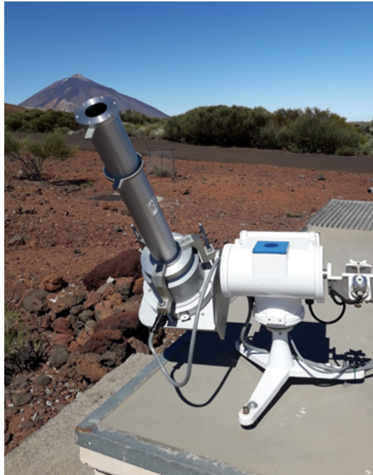
Figure 1. The EKO MS-711 spectroradiometer installed at IZO.
