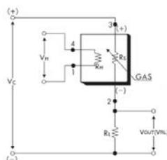
As the reviewer correctly points out, the output voltage ( $V_{RL}$ ) increased with increasing CH<sub>4</sub> concentration. In our setup, we used a load resistor of 10 kOhm and a circuit voltage ( $V_c$ ) of 5 volt.
