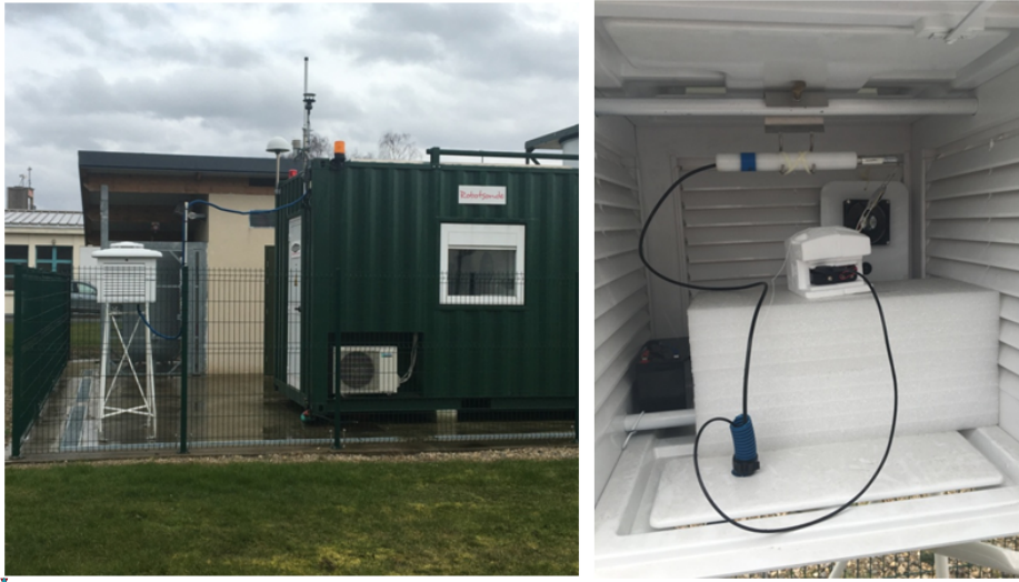
Figure 12: Picture of the meteorological shelter in Trappes (left panel: general view: the meteorological is near the Meteomodem ARL entrance for simplicity reasons, right panel: inside of the meteorological shelter)
