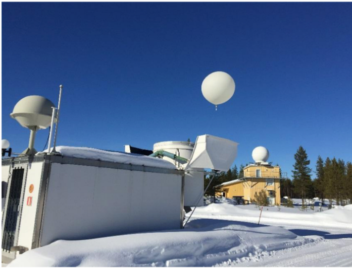
Figure 2: Schematics of the VAISALA Autosonde AS41 system in its most recent configuration (top panel), and photo of the Autosonde system AS15 (bottom panel) operational at the Finnish Meteorological Institute GRUAN site in Sodankylä (WIGOS station identifier=0-20000-0-02836, 67.34 °N, 26.63 °E, 179 m a.s.l., see Vaisala 2018, https://www.vaisala.com/sites/default/files/documents/AUTOSONDE%20AS41%20Datasheet%20B211636EN-A_2%20pages.pdf ).
