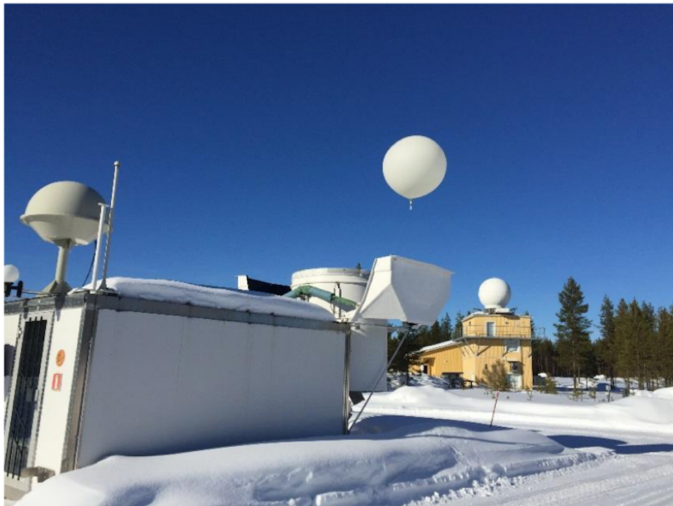
210 Figure 2: Schematics of the VAISALA Autosonde AS41 system in its most recent configuration (top panel), and photo of 211 the Autosonde system AS15 (bottom panel) operational at the Finnish Meteorological Institute GRUAN site in Sodankylä 212 (WIGOS station identifier=0-20000-0-02836, 67.34 °N, 26.63 °E, 179 m a.s.l., see Vaisala 2018, 213 https://www.vaisala.com/sites/default/files/documents/AUTOSONDE%20AS41%20Datasheet%20B211636EN- 214 A_2%20pages.pdf )).
