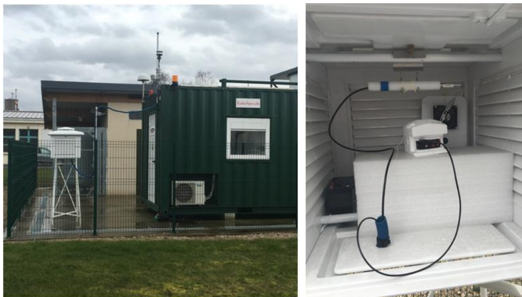
593 Figure 12: Picture of the meteorological shelter in Trappes (left panel: general view: the meteorological is near the 594 Meteomodem ARL entrance for simplicity reasons, right panel: inside of the meteorological shelter)
