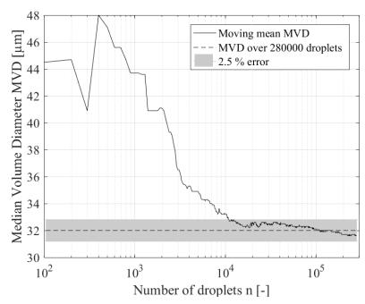
Figure 6: Convergence of MVD over number of droplets at 40 m s<sup>-1</sup> (PDI Run 09/08/17 17:59).
