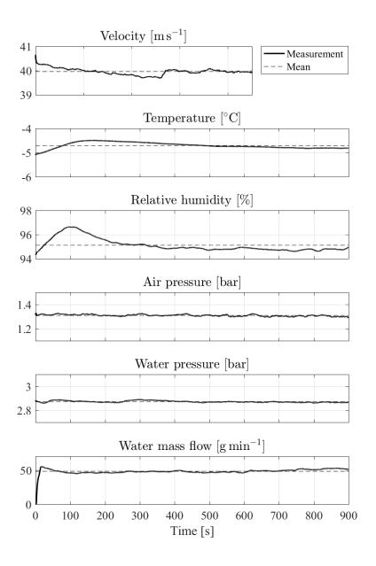
Figure 2: Exemplary stability of the wind tunnel conditions over 15 minutes test duration.
