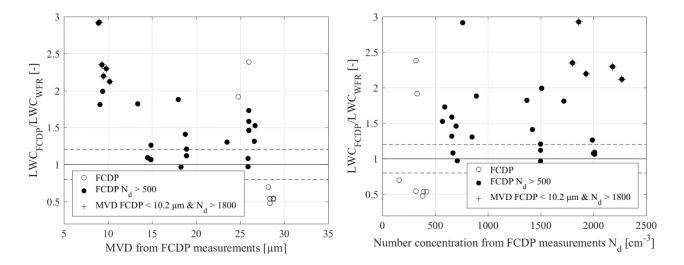
Figure 13: Effect of MVD on LWC measurements from the FCDP (left) and effect of number concentration (right).
