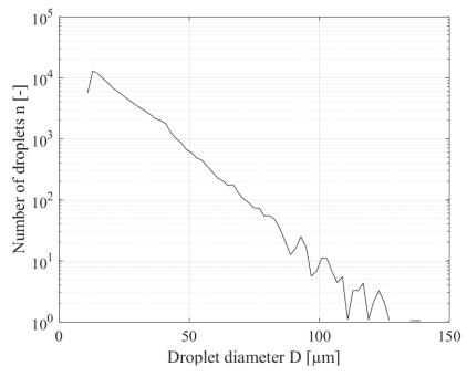
Figure 7: Number of droplets over diameter (PDI Run 18/04/19 18:25), total number of counts >95000.
