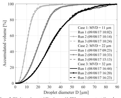
Figure 5: Wind tunnel repeatability shown with PDI measurements at 40 m s<sup>-1</sup>.
