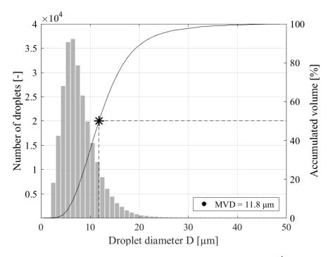
Figure 4: Droplet diameter histogram and cumulative volume curve at 20 m s<sup>-1</sup> (PDI Run 18/04/19 17:19).
