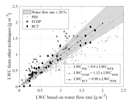
Figure 11: Intercompatrison of LWC based on the water flow rate and measured with the PDI, the FCDP and the RCT.
