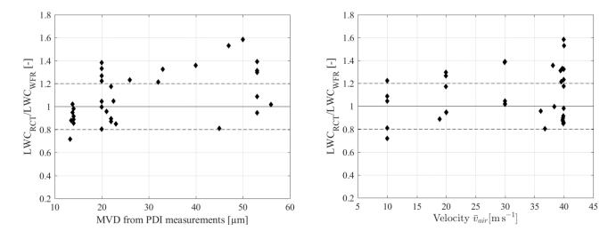
Figure 14: Effect of MVD on LWC measurements from the RCT (left) and effect of air velocity (right).
