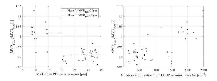
Figure 9: Effect of MVD on droplet size measurements from the FCDP (left) and effect of number concentration (right).
