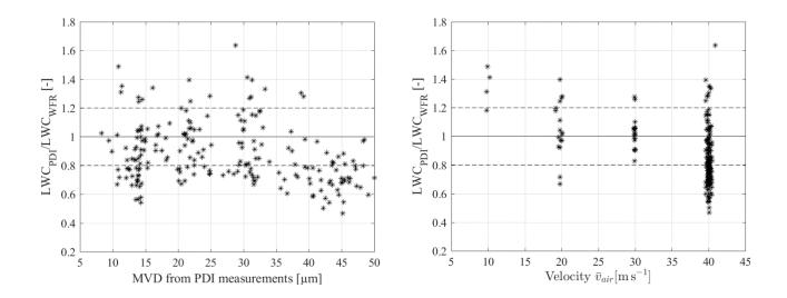
Figure 12: Effect of MVD on LWC measurements from the PDI (left) and effect of air velocity (right).
