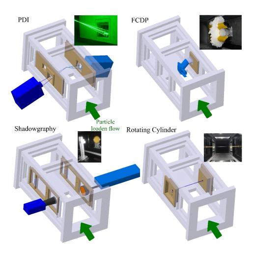
720 Figure 3: Measurement setups in the Braunschweig Icing Wind Tunnel.
