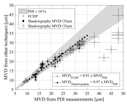
Figure 8: Intercomparison of MVD measured with the PDI, the FCDP and the shadowgraphy.
