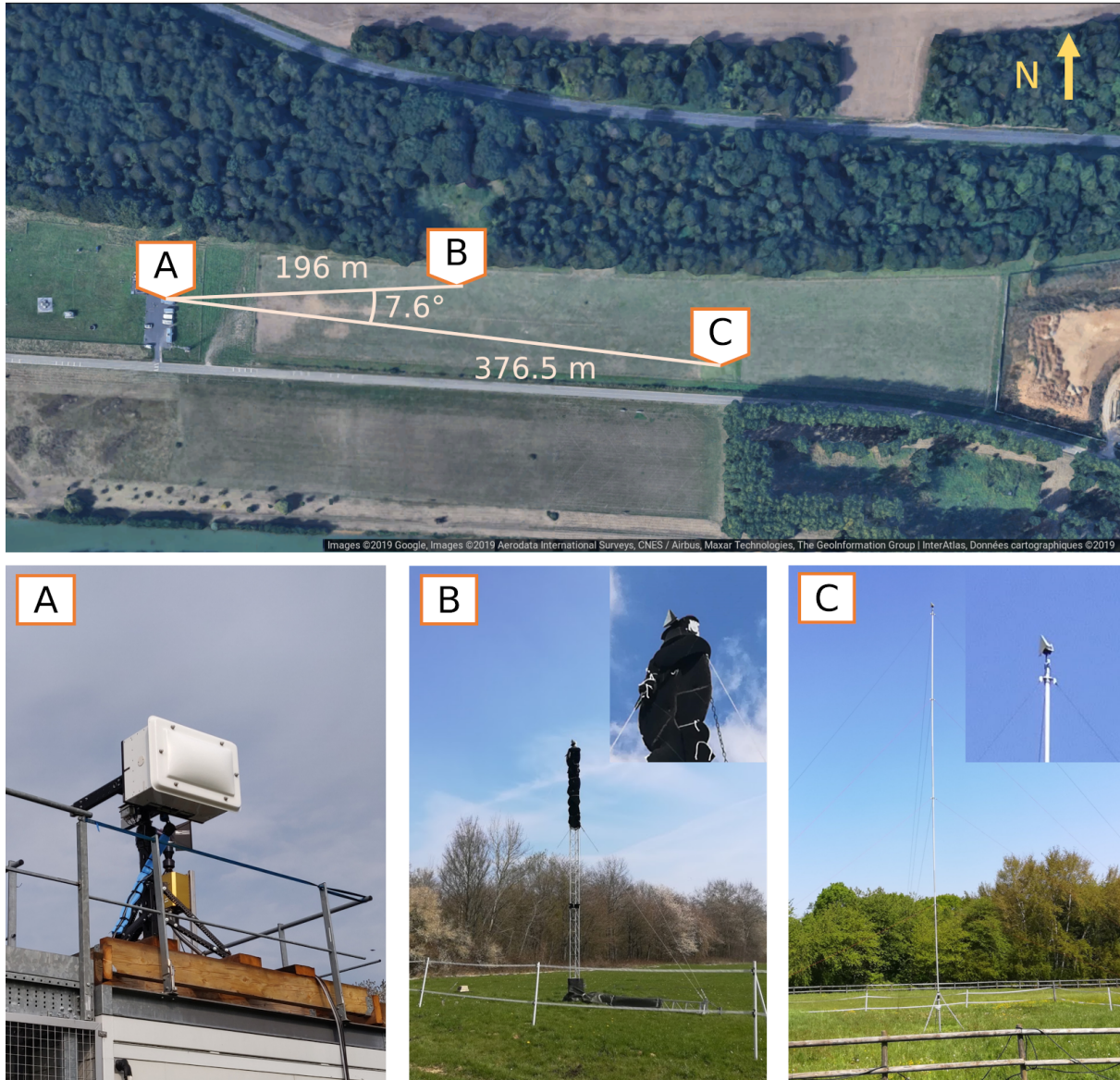
Figure 1. Experimental setup for 2018 and 2019 calibration experiments: (A) Scanning BASTA-Mini radar located in a reinforced platform 5 m above the ground. (B) 10 m mast with a 10 cm triangular trihedral target mounted on a pan-tilt motor with an angular resolution and repeatability better than 0.1^\circ . This mast has microwave absorbing material wrapped to it to reduce its RCS (clutter). The 10 m mast was only installed in the 2019 calibration campaign. (C) 20 m mast with a 20 cm triangular trihedral target. The target aiming is fixed relative to the mast. This mast is used in both 2018 and 2019 calibration campaigns. Angular separation between the masts is enough to sample both targets without mutual interference.
