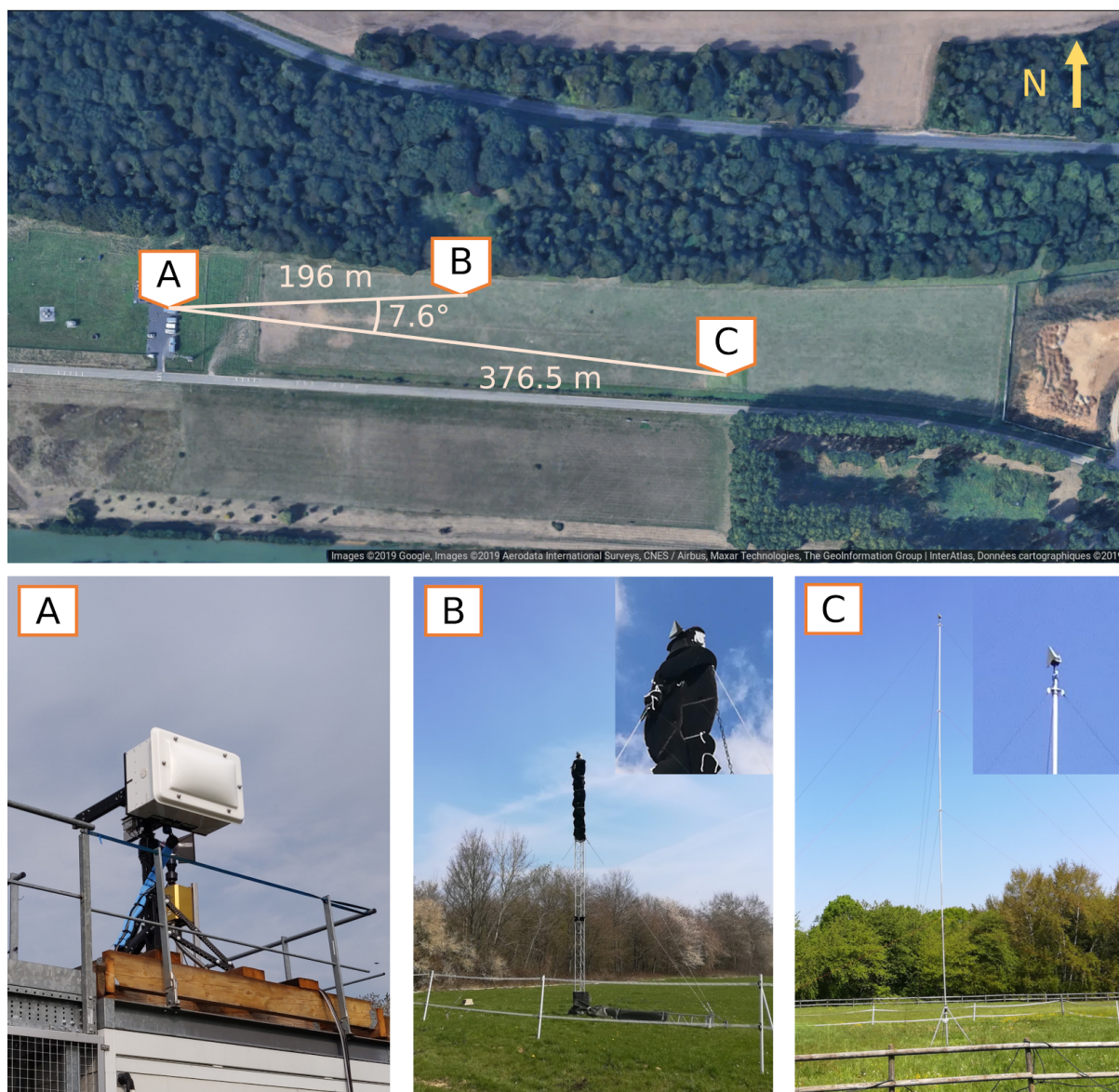
Figure 1. Experimental setup for 2018 and 2019 calibration experiments: (A) Scanning BASTA-Mini radar located in a reinforced platform 5 m above the ground. (B) 10 m mast with a 10 cm triangular trihedral target mounted on a pan-tilt motor with an angular resolution and repeatability better than 0.1^\circ . This mast has microwave absorbing material wrapped to it to reduce its RCS (clutter). The 10 m mast was only installed in the 2019 calibration campaign. (C) 20 m mast with a 20 cm triangular trihedral target. The target aiming is fixed relative to the mast. This mast is used in both 2018 and 2019 calibration campaigns. Angular separation between the masts is enough to sample both targets without mutual interference.
