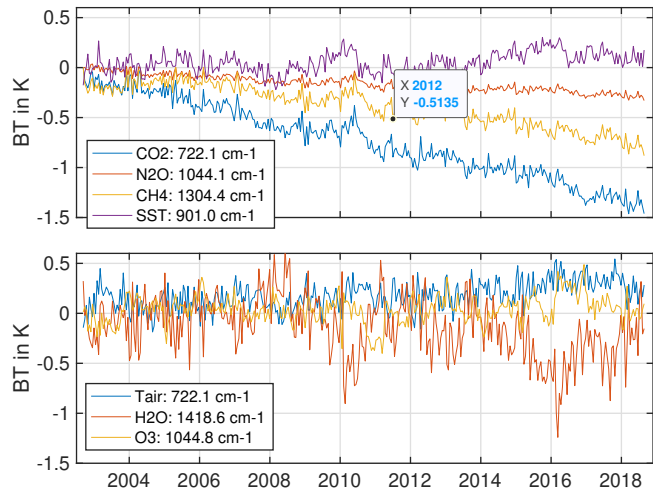
Figure 18. Contribution to the observed BT anomalies caused by the retrieved geophysical anomalies. These are simply the BT Jacobian multiplied by the time-dependent retrieved geophysical anomalies. The BT anomalies in the bottom panel are multiplied by the sum, over all layers, of the retrieved profile anomalies.
