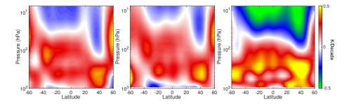
**Figure B4.** Temperature trends from the 16-year data period studied here. Left: ERA-I trends derived directly from the model temperature fields. Middle: Simulated retrievals of the ERA-I trends using radiance anomalies created from the ERA-I fields and our SARTA RTA. Right: Temperature profile trends retrieved from the AIRS observed anomalies. The middle panel simulation assumes that RTA is perfectly accurate.
