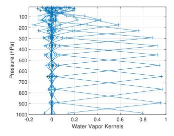
Figure B2. H<sub>2</sub>O kernels for the anomaly retrievals. These are taken from a random day for the zonal bin centered at 28.3°N.
