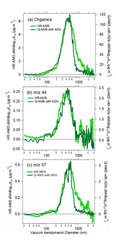
**Figure S3.** Size distributions for organics (a), m/z 44 (b) and m/z 57 (c) from the HR-AMS in bypass (without the ADIc) and the Q-AMS behind the ADIc demonstrating different size cutoffs in the aerodynamic lenses >700 nm in the two instruments.
