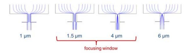
**Figure S1.** Calculated particle trajectories for different particle sizes entering the focusing nozzle of the ADIc. Scale is expanded radially for better visualization.
