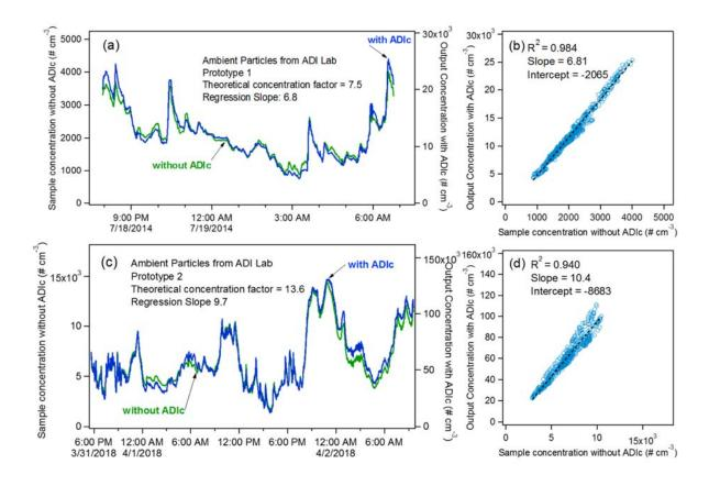
**Figure S2.** Particle number concentrations in the ADIc sample and output flows while sampling laboratory air shown as time series (a, c) and as correlation plots (b, d). Prototype 1 was operating at low flow (a–b) and prototype 2 at high flow (c–d).
