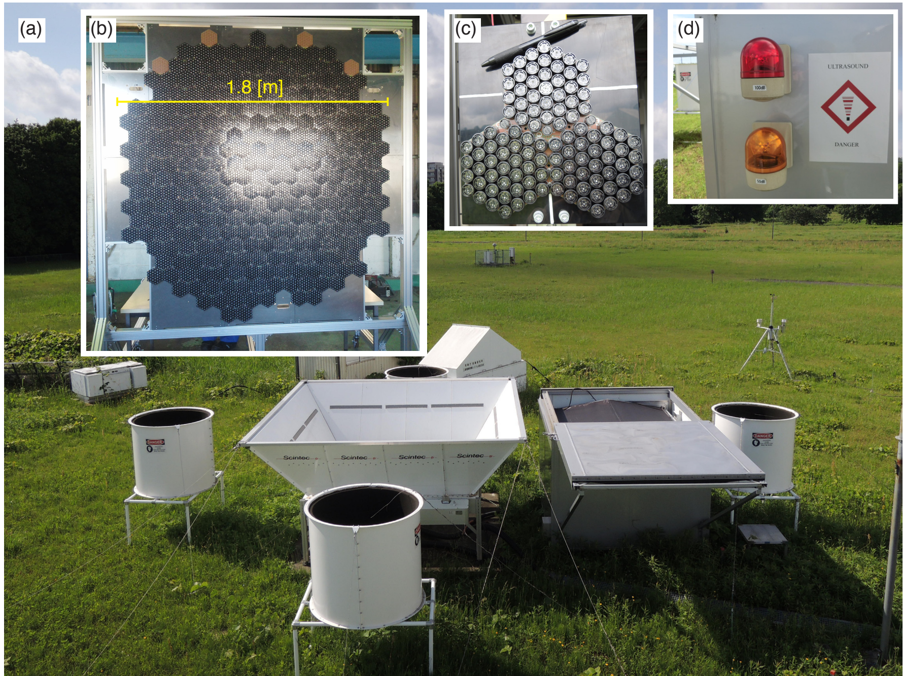
Figure 1. Pictures of (a) LAP-3000 with acoustic speakers and a parametric speaker for RASS, (b) top view, (c) partial expanded view of the parametric speaker, and (d) rotary warning lights on the shed wall. The parametric speaker mounted on top of the shed with a sliding roof is covered with rainproof film in the field, as shown in (a).
