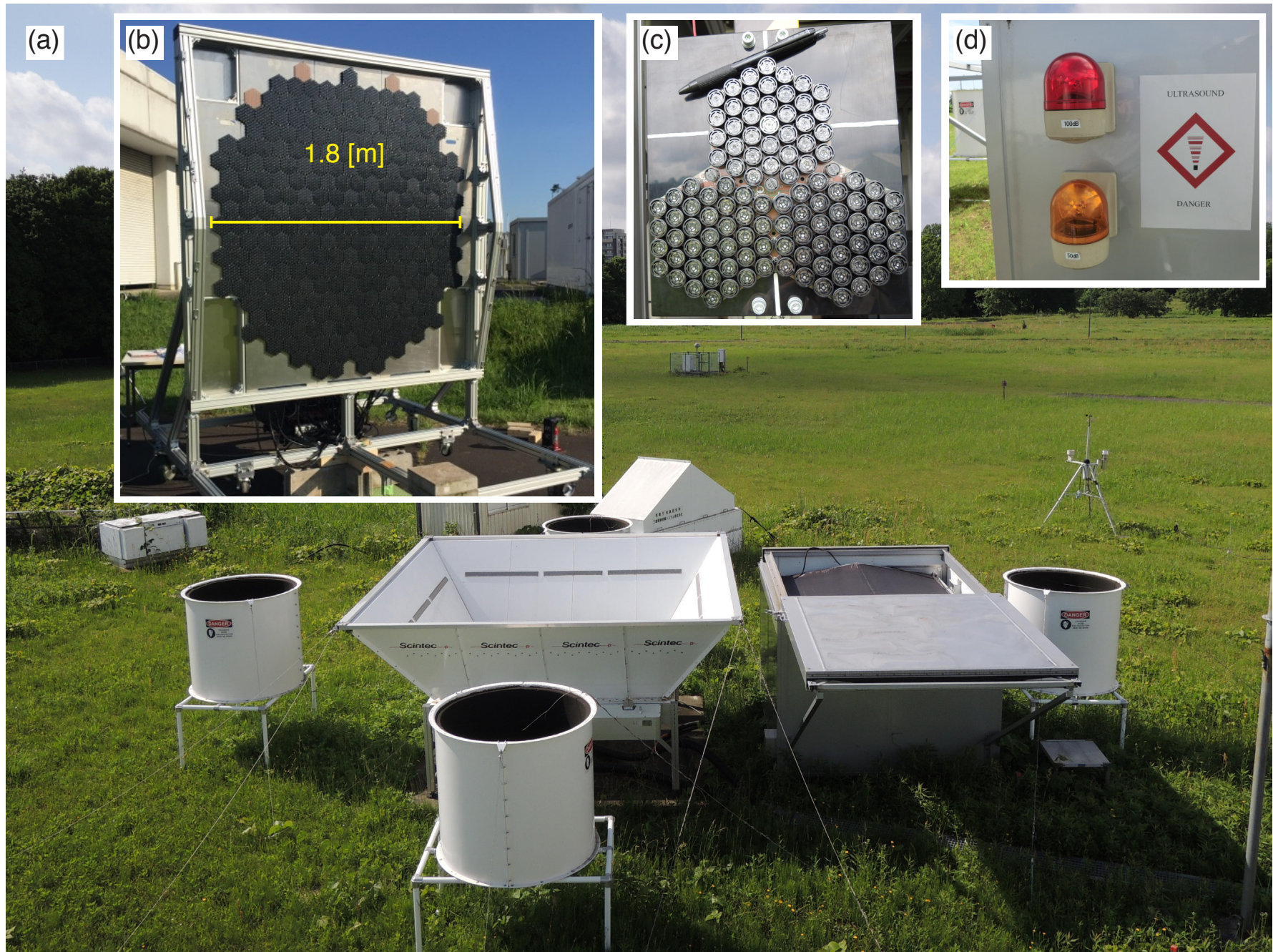
Figure 1. Pictures of (a) LAP-3000 with acoustic speakers and a parametric speaker for RASS, (b) overview on a support frame, (c) partial expanded view of the parametric speaker, and (d) rotary warning lights on the shed wall. The parametric speaker mounted on top of the shed with a sliding roof is covered with rainproof film in the field, as shown in (a).
