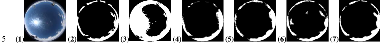
(a) Results of different diurnal cloud segmentation algorithms. (1) Original diurnal ASI image, (2) ground truth of the corresponding ASI image in (1), (3) result of OTSU, (4) result of EFCN-32s, (5) result of EFCN-16s, (6) result of FCN-8s, (7) result of the proposed EFCN-8s.
