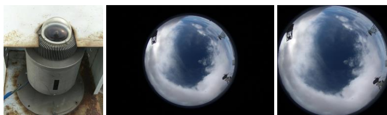
(a) (b) (c) Figure 1: Device of ASI and ASI image. (a) device of ASI including a fisheye lens, an industrial camera and a clear glass cover, (b) original RGB color ASI image (2592×1728 pixels), (c) resized RGB color ASI image of (b) (1408×1408 pixels).
