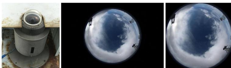
10 **Figure 1: Device of ASI and ASI image. (a) device of ASI including a fisheye lens, an industrial camera and a clear glass cover, (b) original RGB color ASI image (2592×1728 pixels), (c) resized RGB color ASI image of (b) (1408×1408 pixels).**
