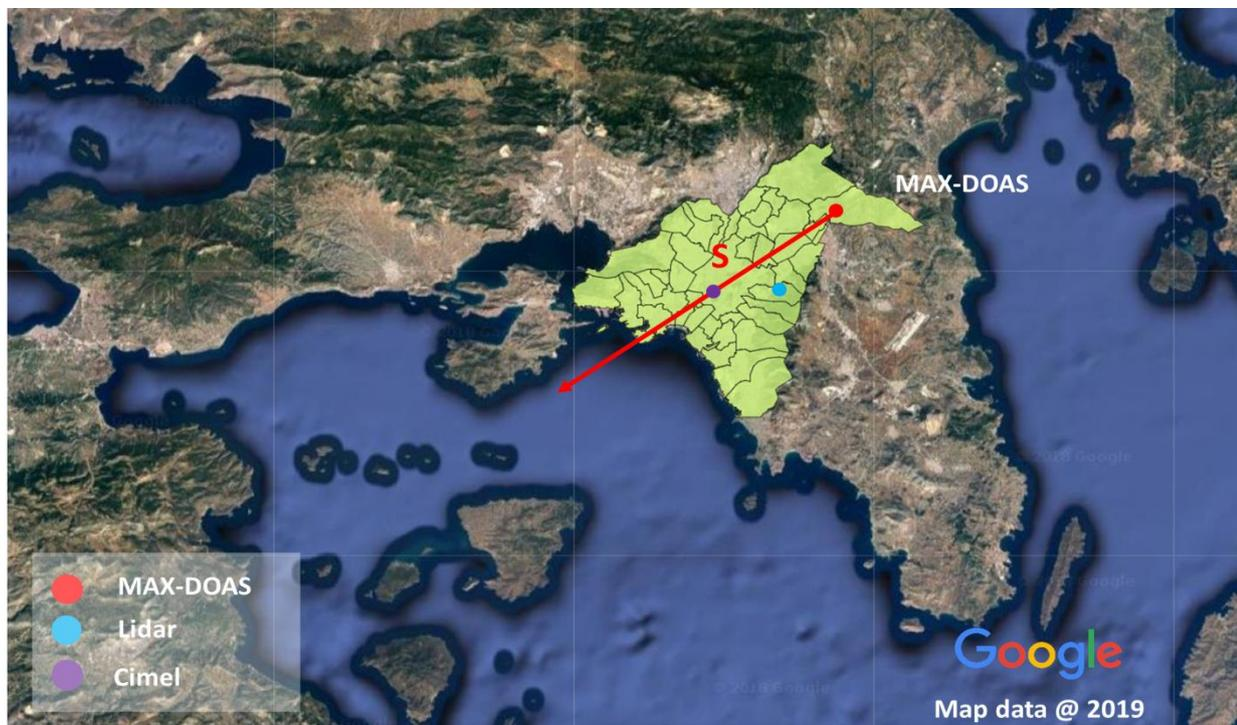
745 **Figure 1: Measurement sites and MAX-DOAS viewing direction (S). The distances between instruments are: MAX-DOAS - sun-photometer (CIMEL) 16 km and MAX-DOAS - lidar 13 km (© Google Maps).**
