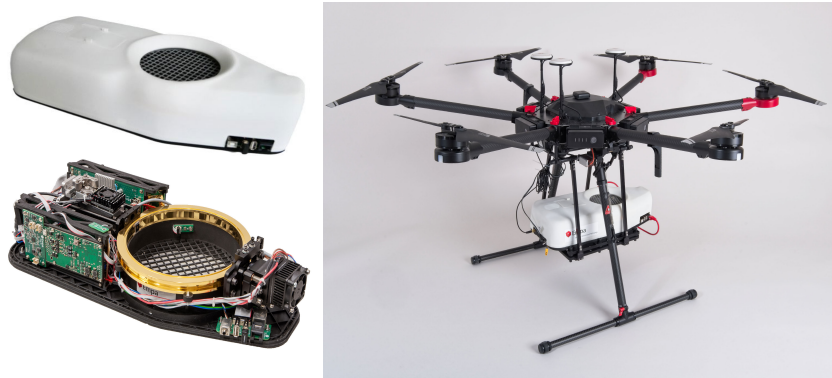
Figure 2. Photograph of the CH 4 laser spectrometer with and without the protecting cover (left). The main building blocks are the TO3-packaged QCL installed on a three-axis stage with additional TEC stabilized heat sink, the SC-MPC with 10 m effective path length, the MCT detector, also with TEC stabilized heat sink, and five PCBs incorporating the hardware electronics: an icw laser driver, a DAQ unit with extension board, a power-supply module, the OEM TEC-board of the detector, and a custom TEC-board for laser and detector heat sinks. The heat sinks of the laser and detector are, in addition, actively air cooled with fans. Picture of the CH 4 sensor installed on the hexacopter (Matrice 600, DJI).
