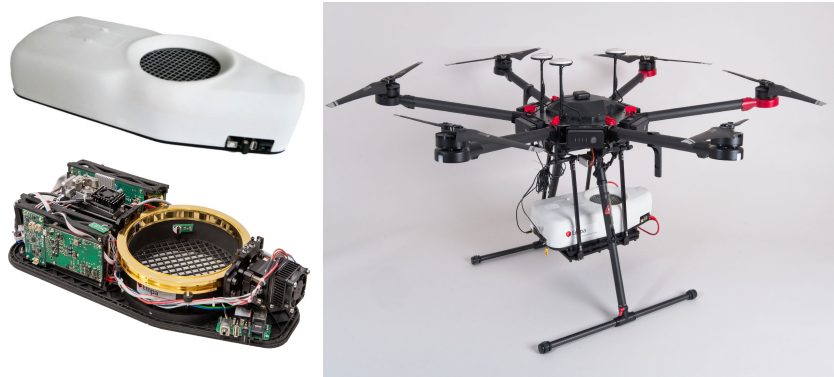
Figure 2. Photograph of the \text{CH}_4 laser spectrometer with and without the protecting cover (left). The main building blocks are the TO3-packaged QCL installed on a three-axis stage with additional TEC stabilized heat sink, the SC-MPC with 10 m effective path length, the MCT detector, also with TEC stabilized heat sink, and five PCBs incorporating the hardware electronics: an icw laser driver, a DAQ unit with extension board, a power-supply module, the OEM TEC-board of the detector, and a custom TEC-board for laser and detector heat sinks. The heat sinks of the laser and detector are, in addition, actively air cooled with fans. Picture of the \text{CH}_4 sensor installed on the hexacopter (Matrice 600, DJI).
