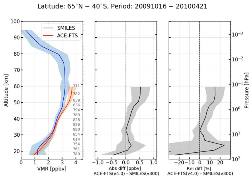
**Figure 8.** Comparison between SMILES and ACE-FTS profiles from October 16, 2009 to April 17, 2010. Left: The mean HCl VMR values (solid lines) and  $1\sigma$  (shaded areas) for SMILES and ACE-FTS. The blue and red lines are the SMILES and ACE-FTS HCl profiles, respectively. Middle: The absolute difference between the SMILES and ACE-FTS profiles calculated using Eq (3). Right: The relative difference between the SMILES and ACE-FTS profiles calculated using Eq (4).
