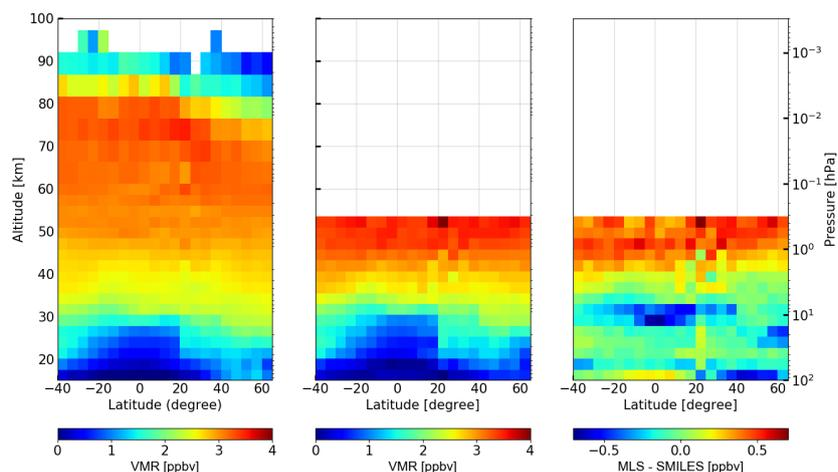
**Figure 6.** Left: SMILES zonal mean HCl profiles versus latitude. Profiles that satisfied coincidence criteria between SMILES and MLS for January 24 – 27, 2010 were used here. Middle: Zonal mean HCl profiles from MLS. Right: The absolute difference of the matched pairs versus latitude.
