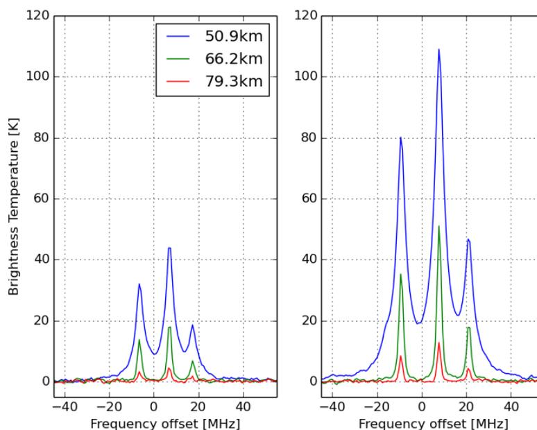
**Figure 2.** Left: An example of the  $\text{H}^{37}\text{Cl}$  spectrum observed by SMILES from a single scan measurement. Tangent heights are approximately 50, 65, and 80 km. Center frequency is 624.98 GHz. Right: An example of the  $\text{H}^{35}\text{Cl}$  spectrum for the same condition as for the  $\text{H}^{37}\text{Cl}$  spectrum. Center frequency is 625.92 GHz.
