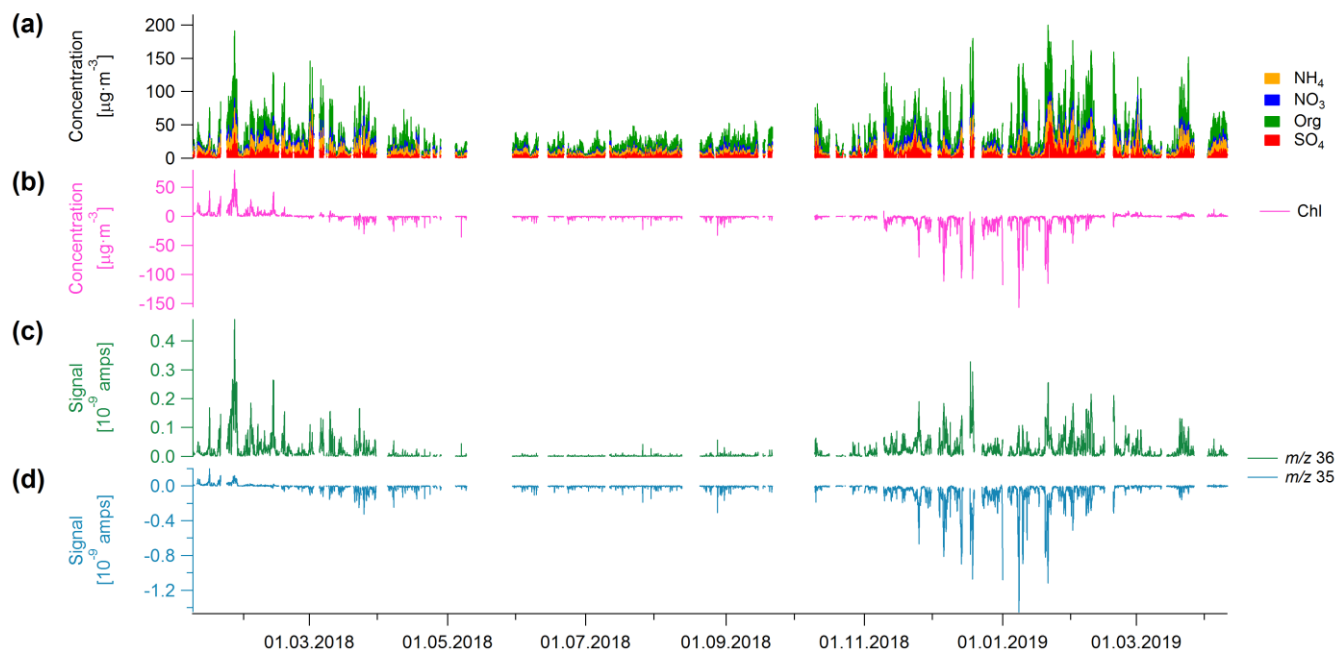
Figure 1. (a) Stacked time series of \text{NH}_4 , \text{NO}_3 , Org and \text{SO}_4 and (b) time series of chloride in \mu\text{g m}^{-3} . Panels (c) and (d) show the time series of m/z 35 and m/z 36 in amps, respectively. The negative chloride signal is driven by the negative m/z 35 signal.
