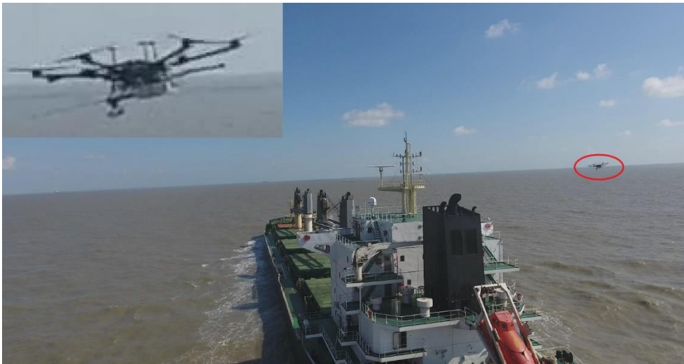
Figure 4. UAV (marked by a red circle) monitoring a ship's emissions in the open sea. The enlarged UAV is shown in the top left corner. This picture was captured by another UAV.
