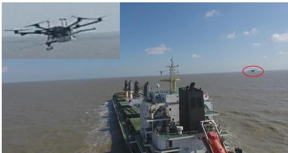
Figure 4. UAV (marked by a red circle) monitoring a ship's emissions in the open sea. An enlarged image of the UAV is shown at the top right. This picture was captured by another UAV.
