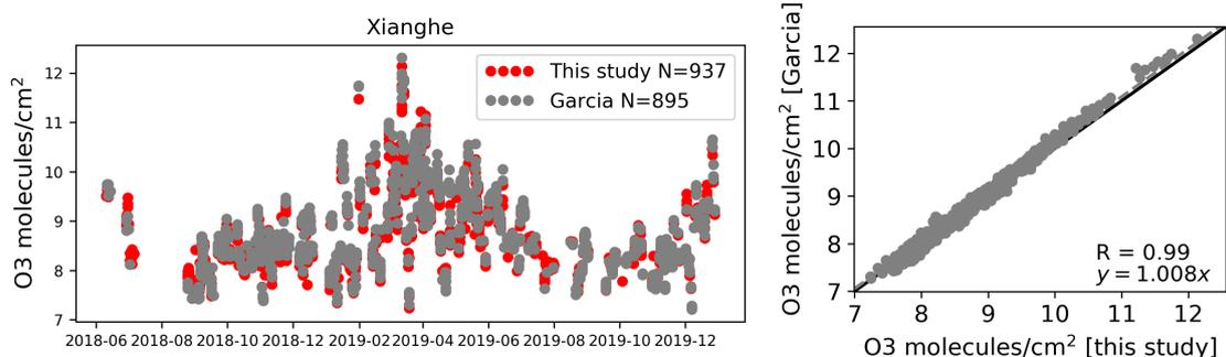
**Figure A2.** [The time series the FTIR retrieved O<sub>3</sub> total column using the windows in this study and García's choice at Xianghe \(left\), together with their correlation \(right\).](#)
