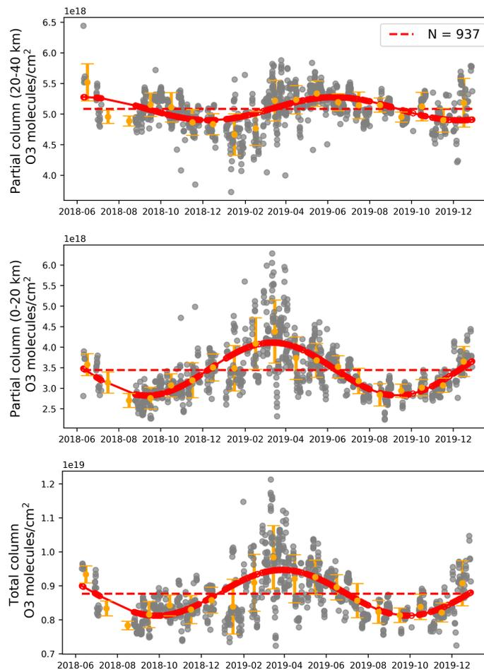
**Figure 3.** The time series of the FTIR retrieved O<sub>3</sub> total column (bottom), as well as the partial column between surface and 20 km (middle) and the partial column between 20 and 40 km (top) from June 2018 to December 2019 at Xianghe. The grey dots are each individual retrieval. The orange dots and errorbars are the monthly means and STDs. The red dashed line is the mean and red solid line is the fitted seasonal variation. N is the measurement number.
