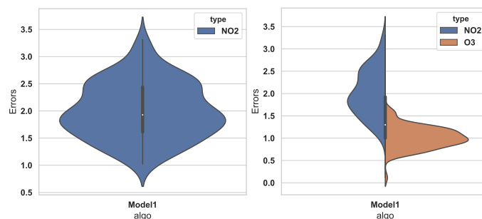
Figure 7. (Interpreting violin plots) Two violin plots based on synthetic error data (i.e. the data does not correspond to any actual model) are shown above. Violin plots display numeric data by showing quartile/percentile information, as well as a rotated kernel density plot to show the distribution of the data. The left figure offers a symmetric violin plot on a single data source (NO 2 calibration in this synthetic example). The thin vertical line in the middle represents the inter-percentile range between the 0.05 and 0.95 percentiles. The thicker and shorter vertical line represents the inter-quartile range between the 0.25 and 0.75 quartiles. The white dot in middle represents the median. The right figure offers a split violin plot that considers two data sources together for ease of comparison.
