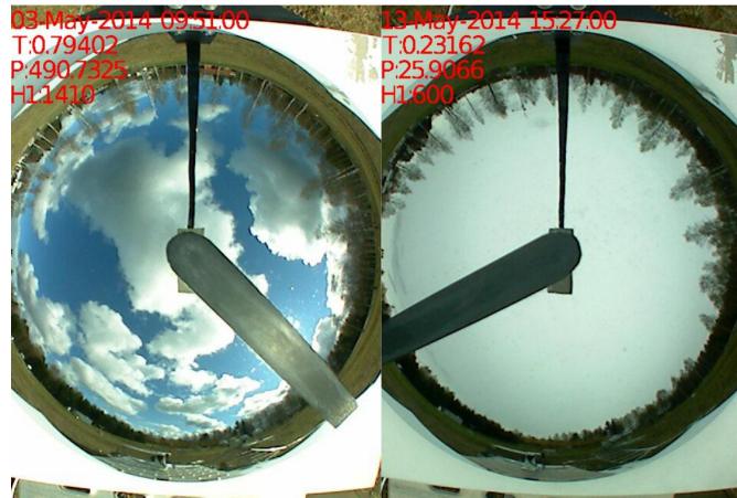
Figure 1. An example of total sky images taken in Hyytiälä that were used when formulating the algorithm. Transmittance, patchiness and the lowest CBH are marked in the figures. Figure courtesy of ARM.
