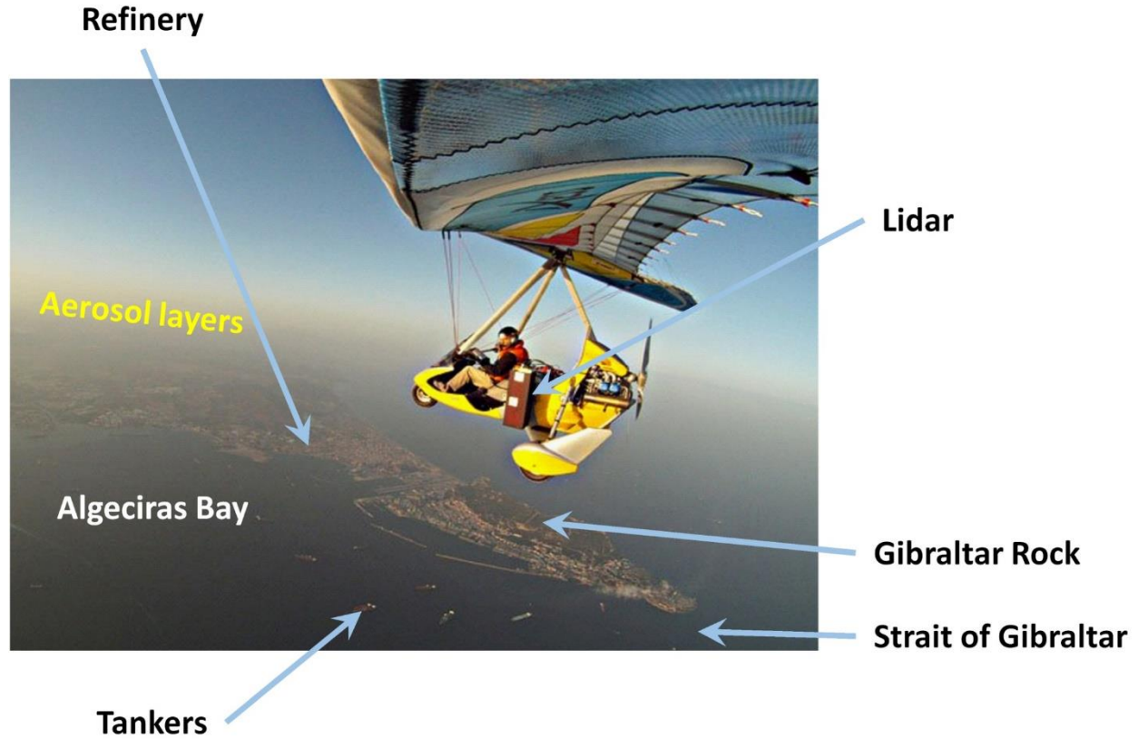
10 Figure 1: ULA above the Strait of Gibraltar. The lidar is located on the left side of the ULA in nadir shooting position. The aerosol layer can be seen in ochre on the horizon of the photo.
