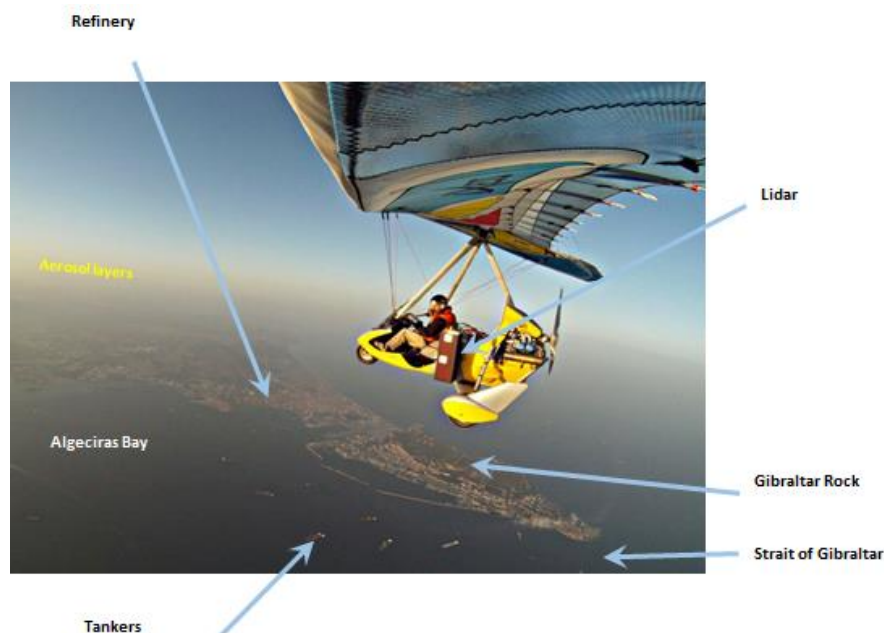
10 Figure 1: ULA above the Strait of Gibraltar. The lidar is located on the left side of the ULA in nadir shooting position. The aerosol layer can be seen in ochre on the horizon of the photo.
