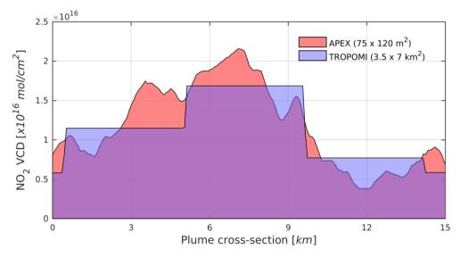
**Figure 12.** APEX and TROPOMI NO<sub>2</sub> VCDs along a southwest-northeast 15 km long cross-section taken perpendicular to the major NO<sub>2</sub> plume retrieved over Antwerp on 29 June 2019. Approximately five TROPOMI pixels and 150 APEX pixels are sampled.
