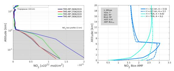
**Figure 3.** (a) Representation of a well-mixed NO<sub>2</sub> box profile of 1 km thickness and TM5-MP NO<sub>2</sub> profiles interpolated over the campaign sites for Flight #1 to #4, and (b) height-dependent box AMFs representing the vertical sensitivity to NO<sub>2</sub>, illustrated for APEX, operating at 6.5 km a.g.l., and TROPOMI, for both a low and high surface reflectance scenario.
