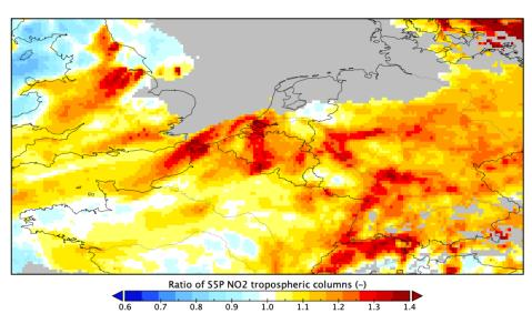
**Figure 2.** Ratio of TROPOMI tropospheric NO<sub>2</sub> columns when using the CAMS-regional a priori NO<sub>2</sub> profiles with respect to TM5-MP a priori profiles over Belgium and neighboring countries on 27 June 2019 (orbit 8826).
