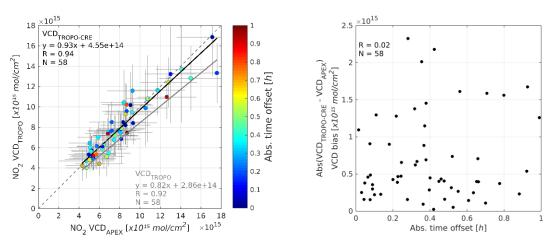
**Figure 10.** (a) Same as Fig. 8.a, but data points are color-coded based on the absolute time offset between TROPOMI overpass and mean acquisition time of APEX retrievals within the TROPOMI pixel, and in (b) the observed NO<sub>2</sub> VCD bias, defined by VCD<sub>TROPO-CRE</sub> – VCD<sub>APEX</sub>, has been plotted against the absolute time offset.
