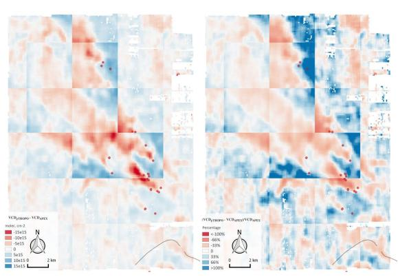
**Figure 14**. (a) The NO<sub>2</sub> VCD bias (VCD<sub>pTROPO</sub> – VCD<sub>APEX</sub>) and (b) relative bias ((VCD<sub>pTROPO</sub> – VCD<sub>APEX</sub>)/VCD<sub>APEX</sub> x 100) for the APEX data set acquired over Antwerp on 29 June 2019. VCD<sub>pTROPO</sub> are pseudo-TROPOMI NO<sub>2</sub> VCDs, constructed by averaging the APEX NO<sub>2</sub> VCDs within grid cells of 4.4 km x 4.4 km.
