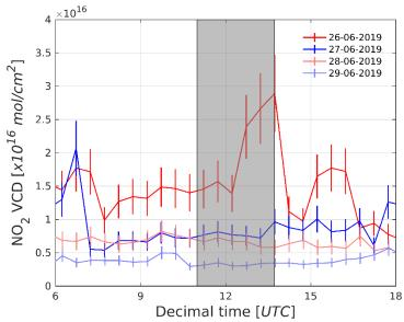
**Figure 11.** Tropospheric NO<sub>2</sub> VCD diurnal variation between 80° sunrise and sunset, retrieved from the Uccle MAX-DOAS station on 26-29 June 2019. The instrument is pointed towards the Brussels city center ( $35^{\circ}$  N). Vertical error bars indicate the NO<sub>2</sub> VCD error for each retrieval. The grey zone indicates the merged APEX flight time (11:00 - 13:44 UTC) for 26 to 29 June.
