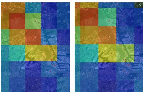
**Figure 13**. (a) APEX NO<sub>2</sub> VCD grid retrieved over Antwerp on 29 June, at 0.1 km x 0.1 km resolution, and the computed pseudo-satellite NO<sub>2</sub> VCDs grids at (b) 1 km x 1 km, (c) 4.4 km x 4.4 km, and (d) 5 km x 5 km, respectively. In the 4 plots, the same color-code is applied with the legend provided in (a) ( $\bigcirc$  Google Maps).
