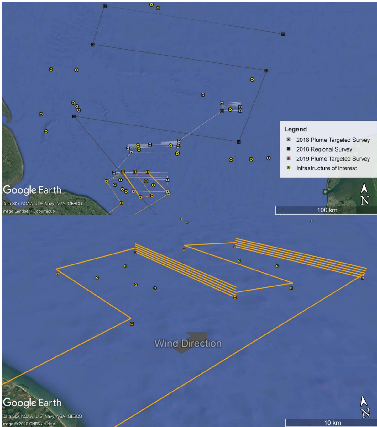
Figure 3: [ top Top panel] flight patterns showing the regional and plume capture styles of flight deployed between 2018 and 2019, alongside infrastructure of interest (such as drilling rigs, gas distribution platforms or production platforms). [ bottom Bottom panel] a 2019 plume sampling survey showing idealised stacked transects in the 2D plane downwind of infrastructure of interest.
