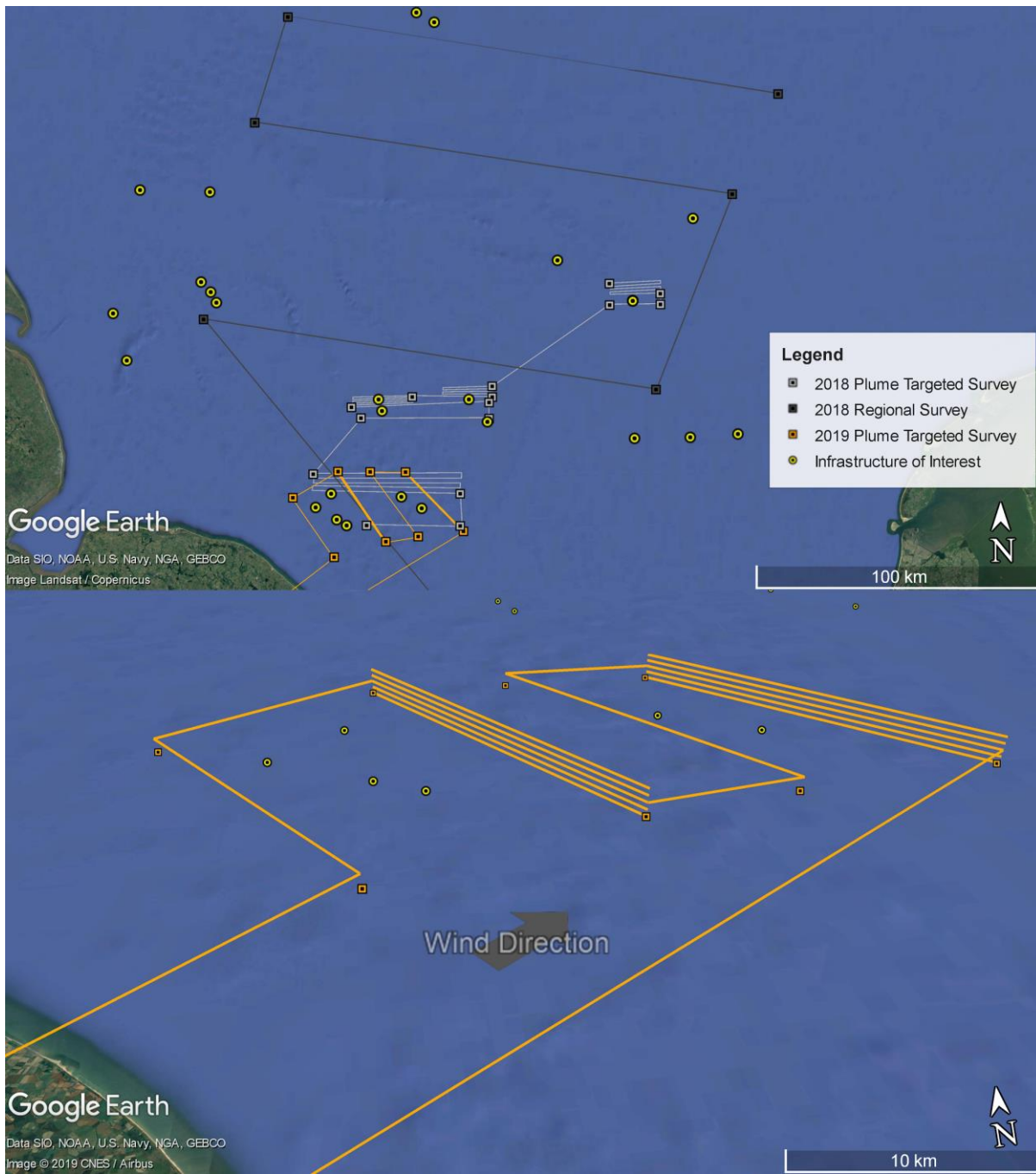
Figure 3: [Top panel] flight patterns showing the regional and plume capture styles of flight deployed between 2018 and 2019, alongside infrastructure of interest (such as drilling rigs, gas distribution platforms or production platforms). [Bottom panel] a 2019 plume sampling survey showing idealised stacked transects in the 2D plane downwind of infrastructure of interest.
