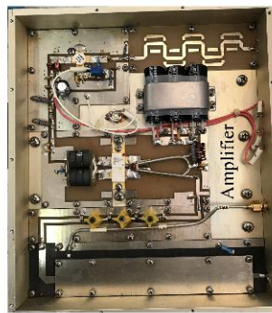
Figure 5. Block diagram (a) and photograph (b) of the small TR module.
