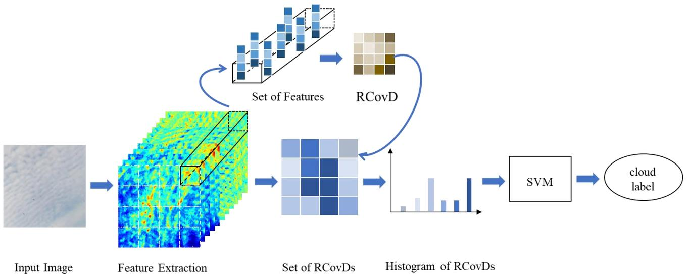
**Figure 1: Pipeline of the proposed cloud classification method. Multiple pixel-level features are firstly extracted from the cloud image blocks to form RCovDs, then the histogram representation of RCovDs are obtained by Riemannian BoF, finally, the cloud type is predicted by multiclass SVM.**
