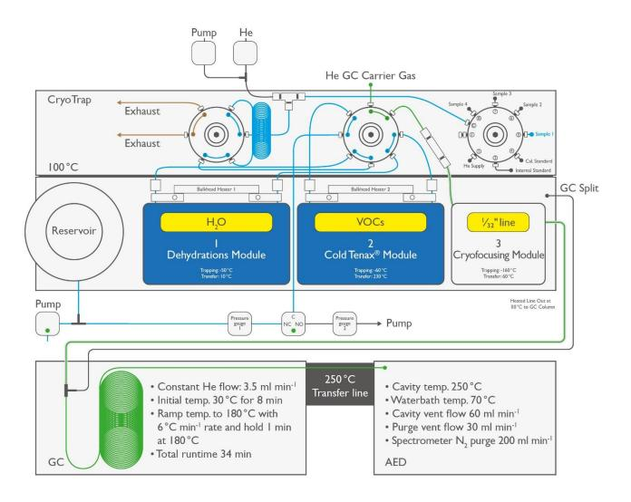
Figure 1: Schematic overview of instrumental setup, CryoTrap-GC-AED.
