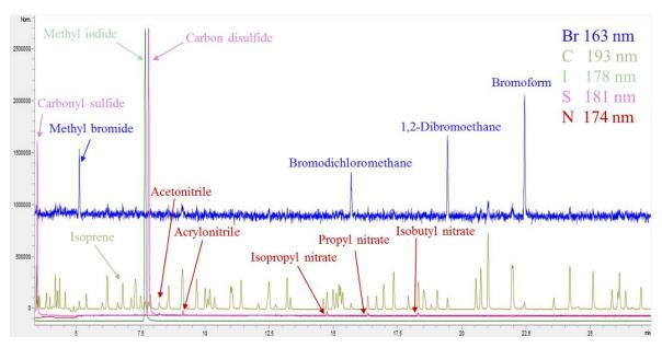
Figure 2: Example CryoTrap-GC-AED normalized multi-element overlay chromatogram of  $\sim$ 250 pptv 84 component Apel-Riemer-2015 gas calibration standard.
