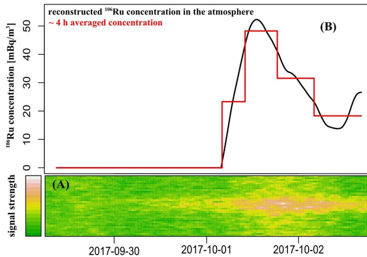
**Figure 2.** The response of the AMARA system to the  $^{106}\text{Ru}$  contamination passing over during the corresponding sampling interval; A) the  $^{106}\text{Ru}$  signal increase in the (615 - 630) keV energy region after subtracting the radon background; B) the example reconstructed real-time  $^{106}\text{Ru}$  concentration and its 4-hour averaged values which corresponds to the CEGAM time resolution .
