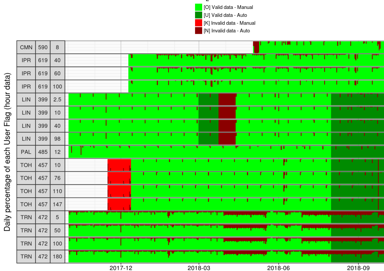
Figure 3. Example of data validation for six stations: CMN (Monte Cimone, Italy), IPR (Ispra, Italy), LIN (Lindenberg, Germany), PAL (Pallas, Finland), TOH (Torfhaus, Germany), TRN (Trainou, France). Dark colored data are data controlled by the software only. Light colored data are controlled by the PI. Green is valid, red invalid. On the left, the first column shows the station acronym, the second column the ICOS ID of the instrument and the third the sampling height.
