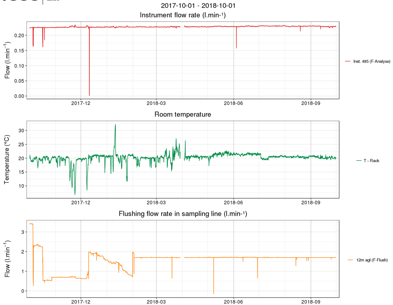
Figure 10. One year of diagnostic parameters at Pallas station (PAL). From top to bottom: instrument flow rate, room temperature and sampling line flushing flow rate.
