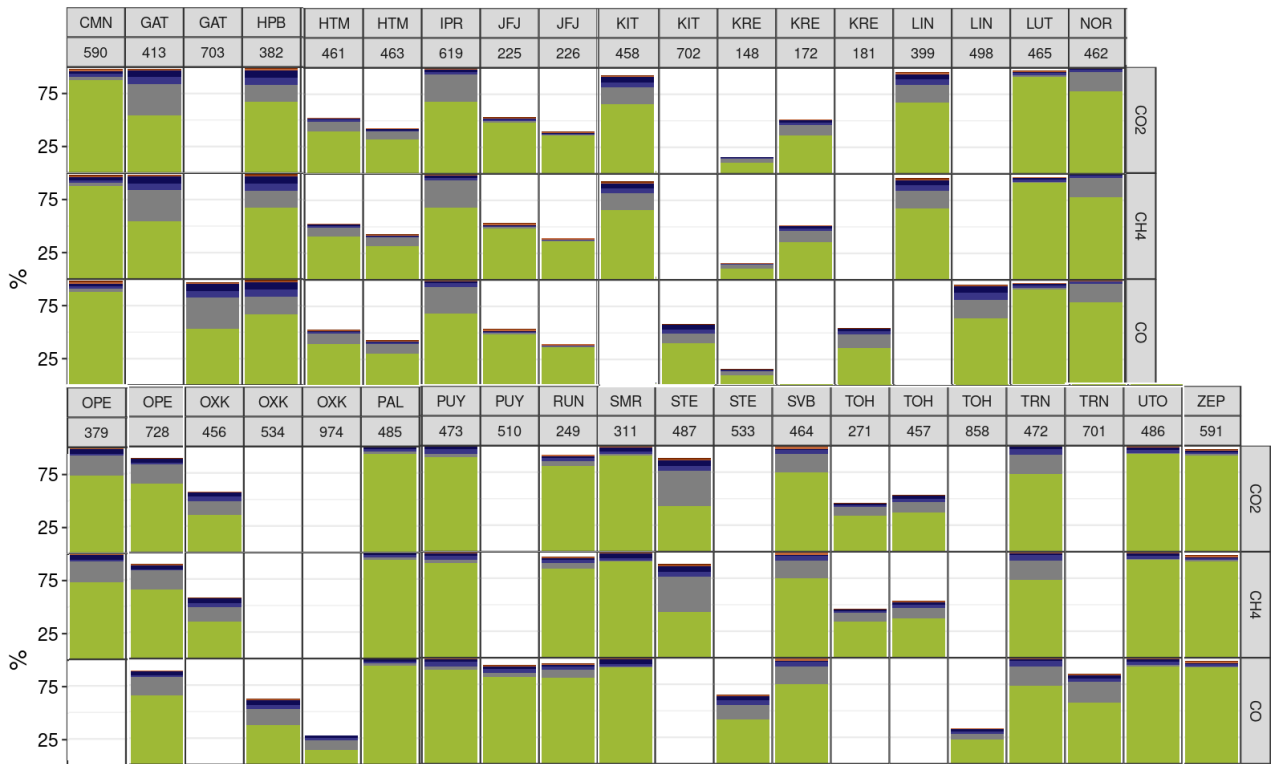
Figure 14. Data distribution between ambient air, target and calibration gases for the 23 stations for CO 2 , CH 4 and CO over the past year. Calibration is in red, target in blue and air in green/gray. Gray and darker color are invalid data. 100% is reached when data are available for the full year. For some stations, two instruments are used to measure CO 2 , CH 4 and CO (see their ICOS ID on the second line). For other, due to instrumental failure, a new instrument has replaced the previous one. See Table 3 for the acronyms and more details about each station.
