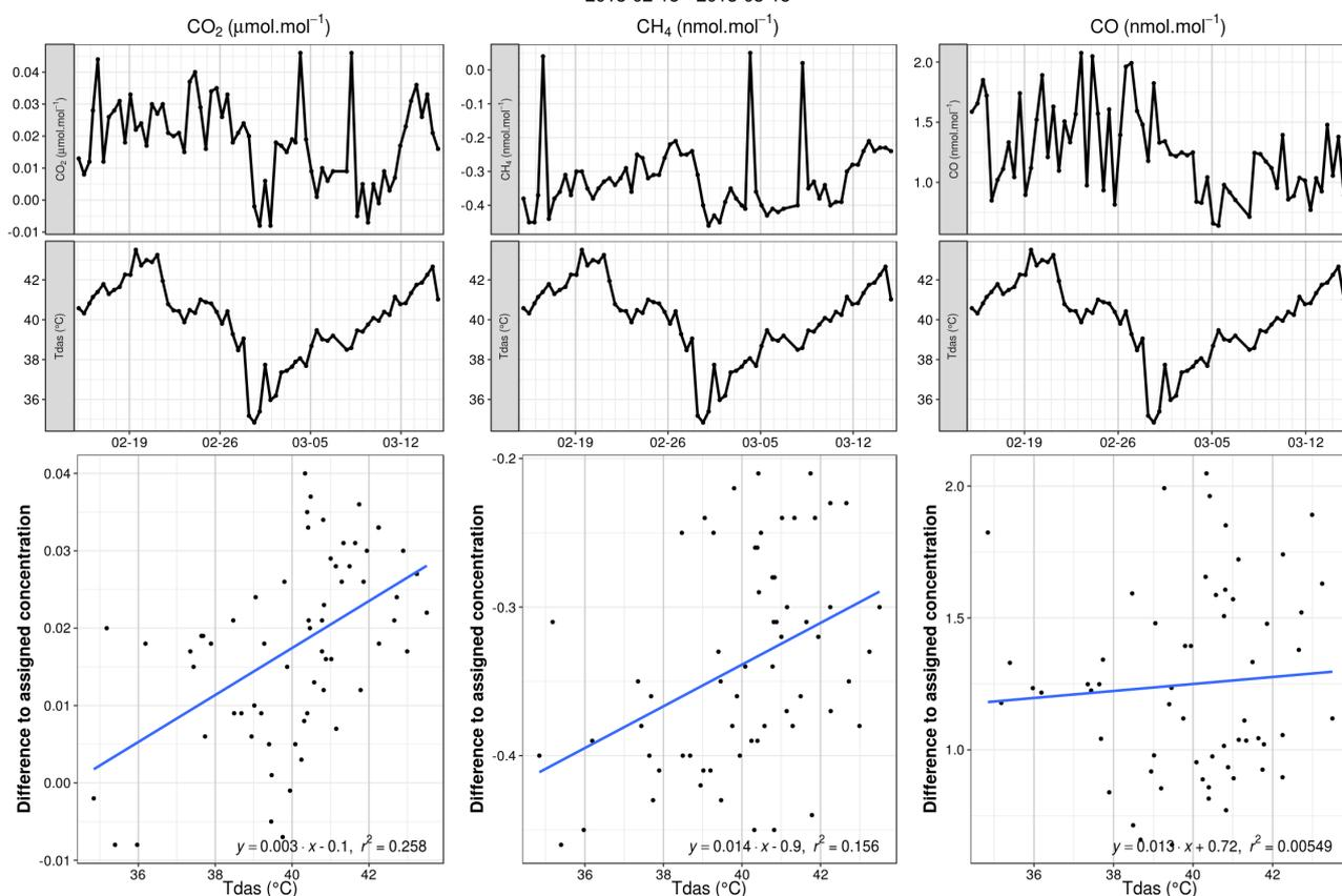
**Figure 8.** Temperature influence on the measurements. On top, greenhouse gas and instrument temperature (Tdas) measurements against time. On the bottom, greenhouse gas measurements against instrument temperature. In most of the case, no dependencies are seen.
