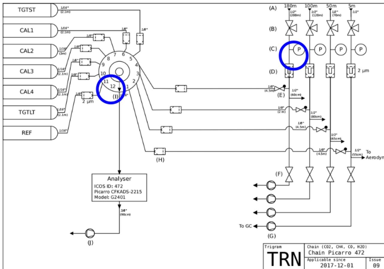
**Figure 2.** Station schematics with injection points in blue for the shelter test.
