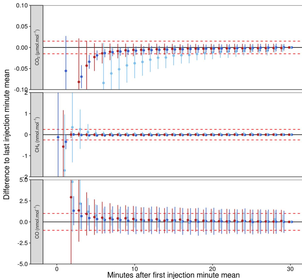
**Figure 5.** Difference between the last injection minute averaged data point and the rest of the injection for cylinder samples. All the injections over the last six months are averaged. Short-term target is in dark blue, long-term target in light blue and calibration in red. Red dashed lines show the thresholds. Vertical lines on each point show the minute standard deviation.
