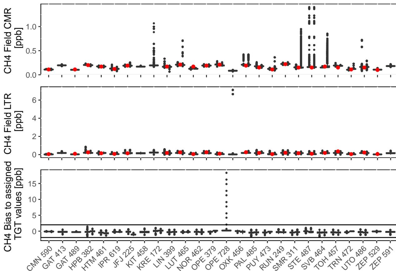
**Figure 17.** Uncertainties and bias to the short-term target for CH<sub>4</sub> defined as in Figure 13. In red, the minute CMR and LTR from the MLab initial tests are shown. The left box (pink) is calculated using data from the year prior to labeling. The right box (blue) is calculated using data from March 2019 to March 2020. The x-axis shows the site trigram and the ICOS ID of the analyzer. The black lines in the bias plot show the WMO compatibility goals.
