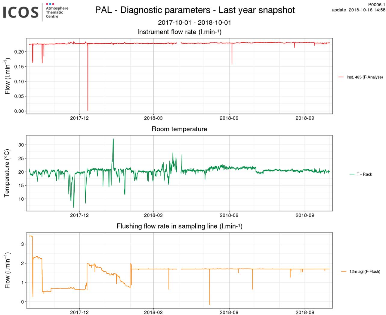
**Figure 10.** One year of diagnostic parameters. From top to bottom: instrument flow rate, room temperature and sampling line flushing flow rate.
