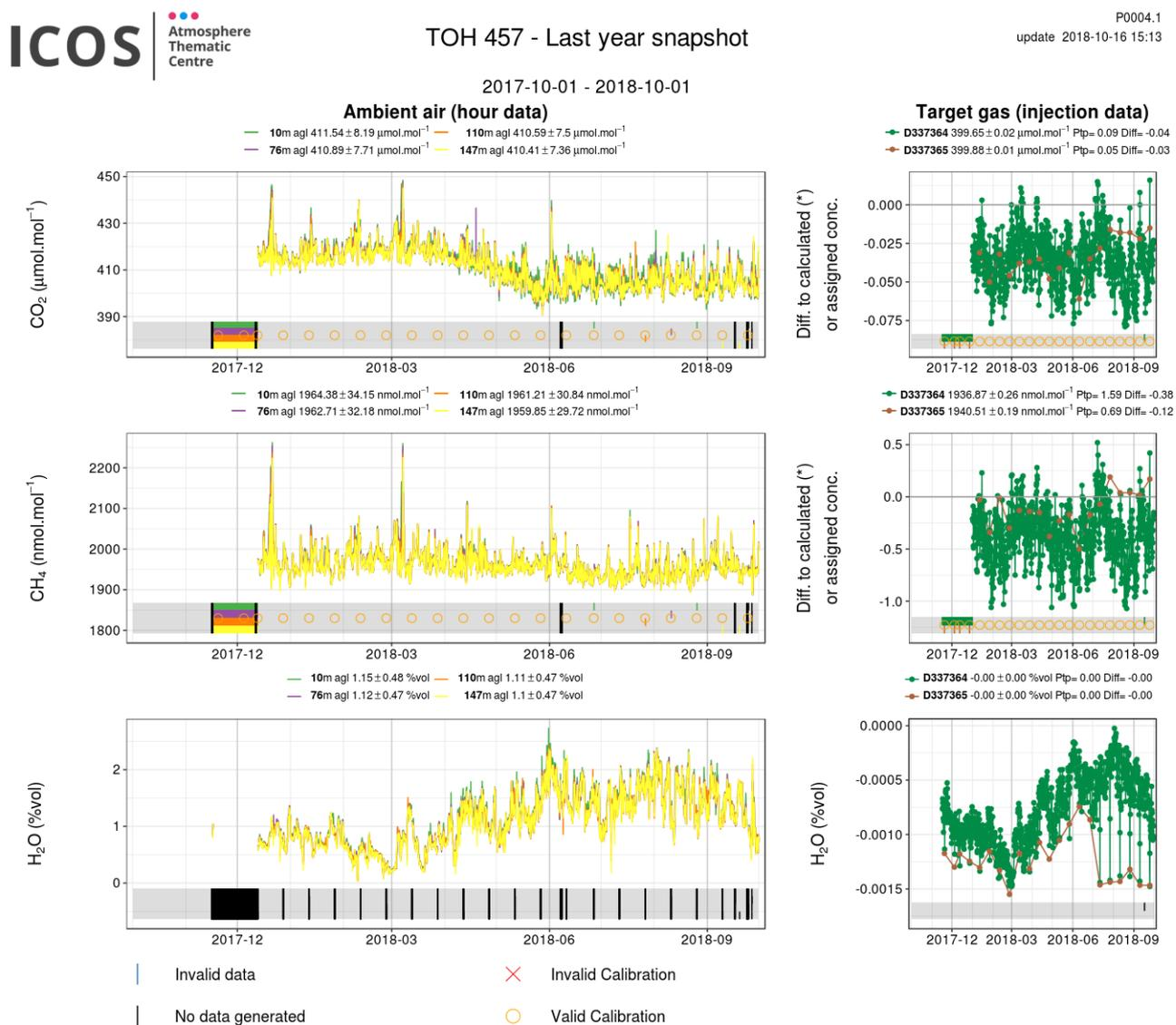
**Figure 11.** One year of hourly averaged greenhouse gas measurements. The different levels and targets are plotted with different colors. Ambient air is plotted on the left, target measurements on the right. Calibration are shown with orange circles. Invalid data are shown at the bottom.
