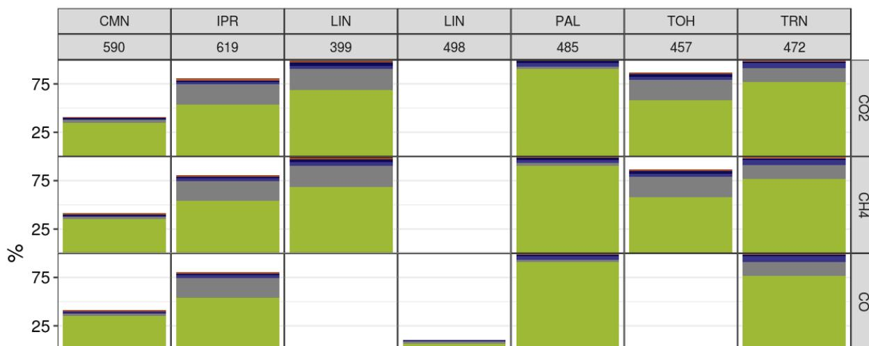
**Figure 4.** Data distribution between ambient air, target and calibration gases for the same 6 stations as Figure 3 for CO<sub>2</sub>, CH<sub>4</sub>, CO. Calibration is in red, target in blue and air in green/gray. Gray and darker color are invalid data. 100% is reached when data are available for the full year.
