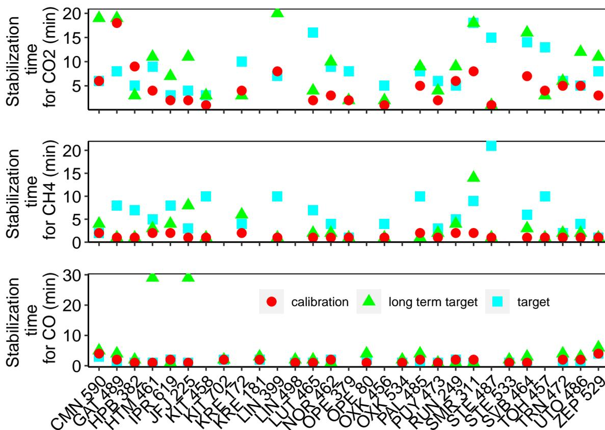
**Figure 15.** Stabilization time for CO<sub>2</sub>, CH<sub>4</sub> and CO at the 23 stations at the time of the labeling. Red show the calibration, green the long-term target and blue the short term-target. On the x-axis is shown the trigram of the station and the ICOS ID of the analyzer. Data from CRDS and OA-ICOS analyzers are shown.
