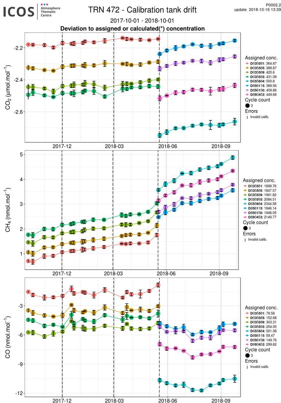
**Figure 6.** Evolution of the analyzer output when measuring different calibration gases with respect to the assigned values over a year. Each calibration cylinder is shown with a different color. Assigned values are indicated on the right.
