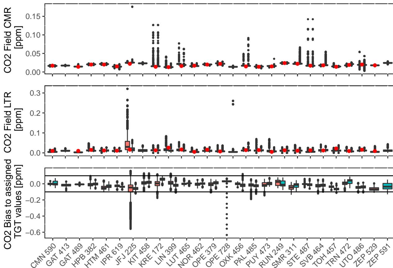
**Figure 16.** Uncertainties and bias to the short-term target for CO<sub>2</sub> defined as in Figure 13. In red, the minute CMR and LTR from the MLab initial tests are shown. The left box (pink) is calculated using data from the year prior to labeling. The right box (blue) is calculated using data from March 2019 to March 2020. The x-axis shows the site trigram and ICOS ID of the analyzer. The black lines in the bias plot show the WMO compatibility goals.
