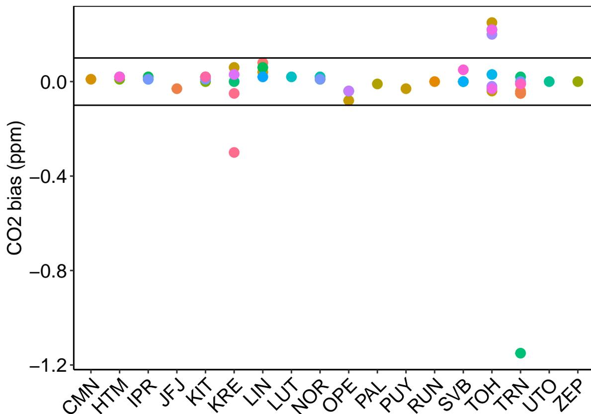
**Figure 19.** CO<sub>2</sub> difference between the reference injection and the injection before the shelter first element. The different colors show the difference at each sampling levels. Dots of the same colors indicate that several tests have been performed. The black lines show the WMO compatibility goals.
