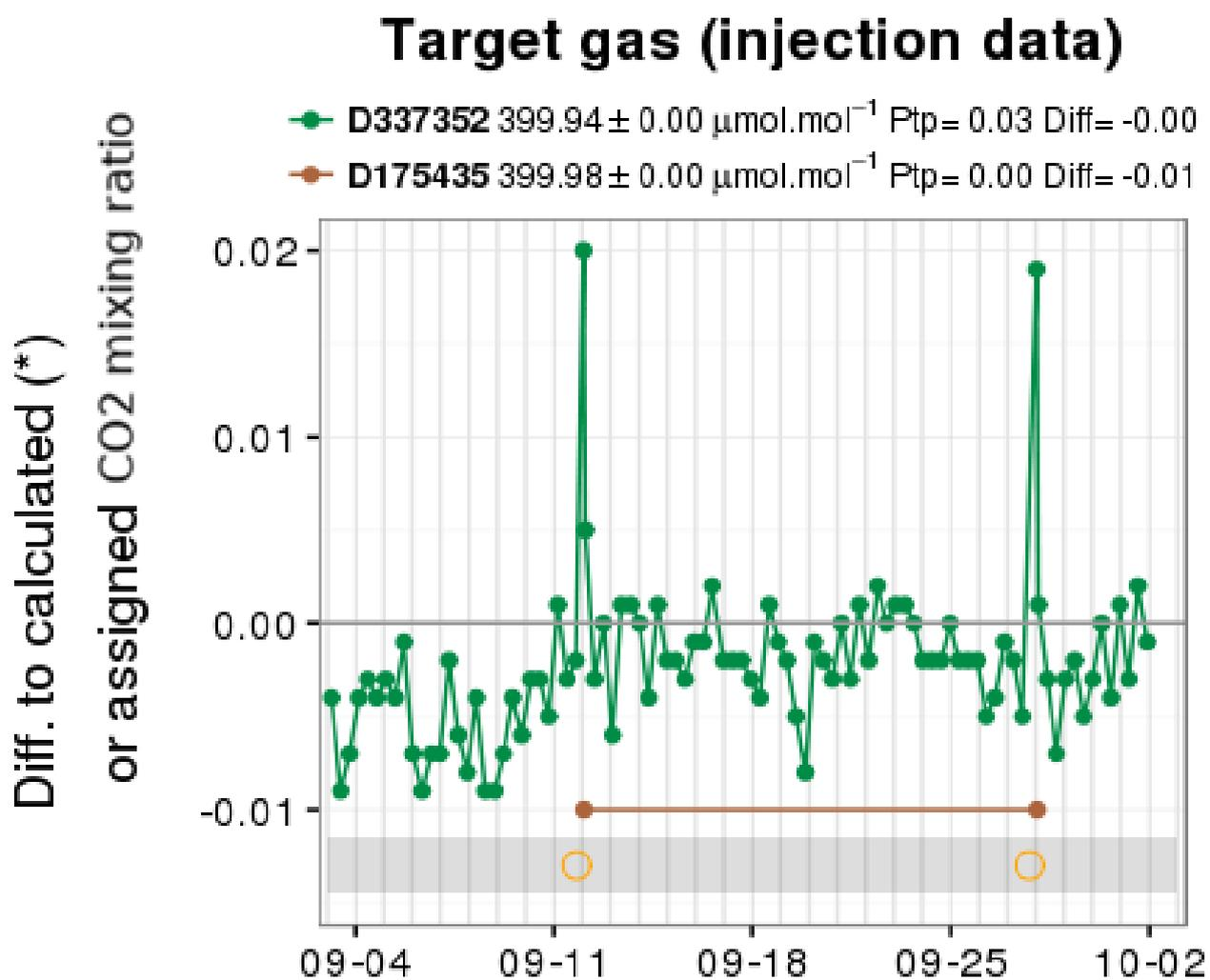
**Figure 1.** One month of target gas injections for CO<sub>2</sub> (ppm). Short term target is plotted in green, long term is in brown. The calibration dates are shown by the light orange circles. Difference to the assigned values is shown. Average values, point-to-point variability and difference to the assigned value are written up top.
