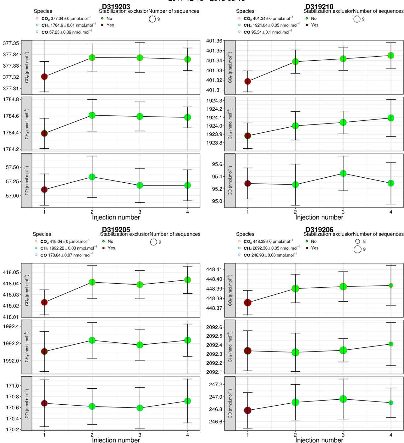
**Figure 7.** Average of each cycle injection for the last calibrations over three months. Green dots are data used for the calibration correction, red is rejected for stabilization. The number of calibrations is shown on the top right. Assigned values are on the top left.
