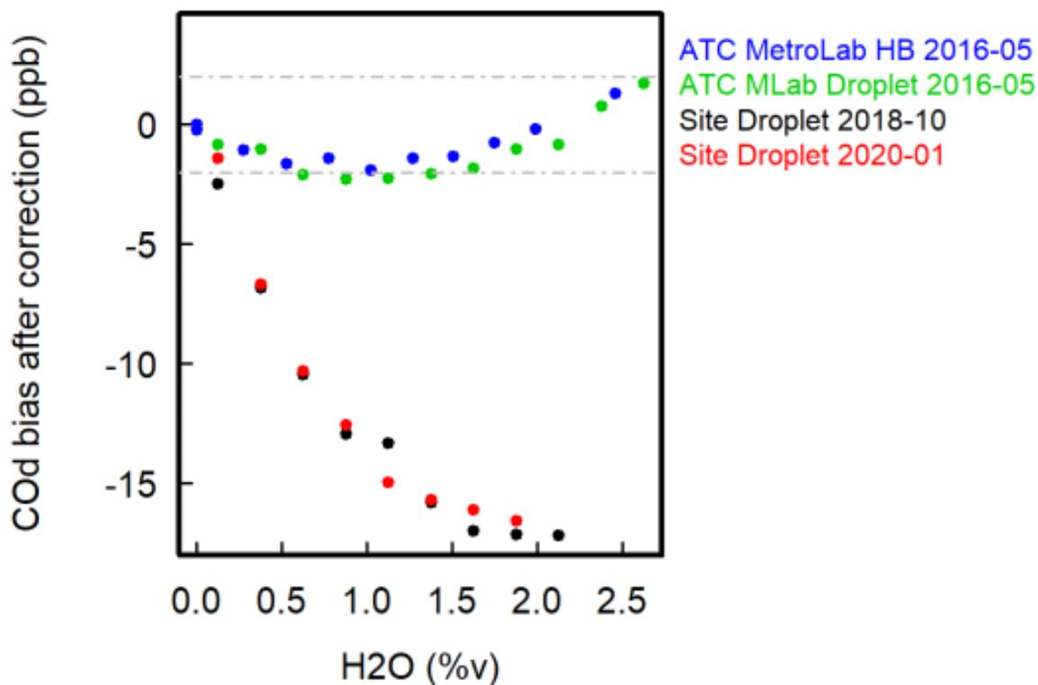
**Figure 20.** Example of water vapor correction assessment over time for CO.
