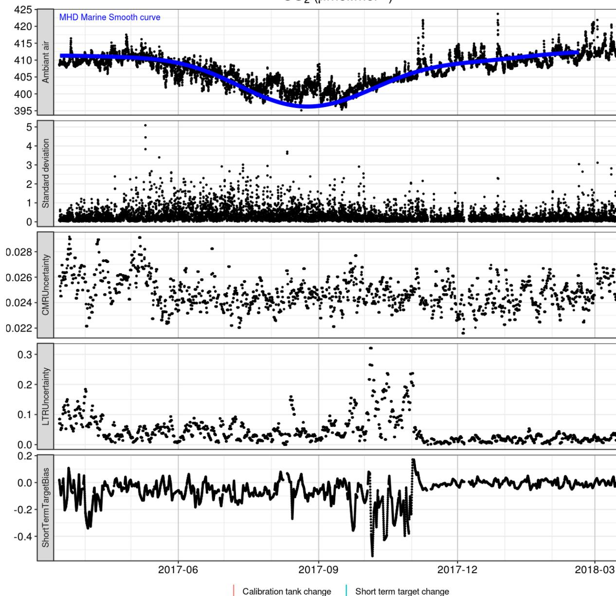
**Figure 12.** Last year of greenhouse gas measurements along with estimated uncertainties. Continuous measurement repeatability (CMR) and long-term repeatability (LTR) are calculated as in Yver Kwok et al. (2015). The short-term target bias is calculated as the difference between the hourly average of the short-term target injections and the value assigned by the FCL-CAL.
