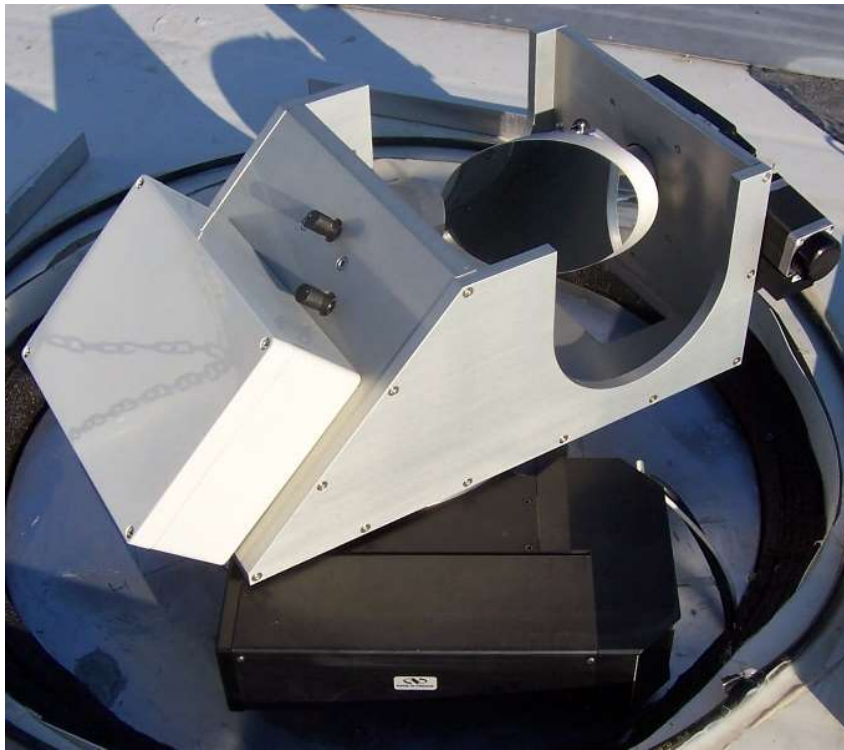
Figure 2: The completed tracker (Lauder, New Zealand) installed at roof level, on a tower mounted to the laboratory concrete floor.
