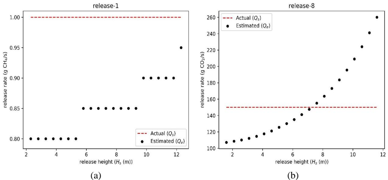
Figure R2: Estimates of the release rates with varying release heights for (a) release-1 (CH<sub>4</sub>) and (b) release-8 (CO<sub>2</sub>). The first estimates of the release rates correspond to the actual source heights. The dotted red lines represent the actual release rates.
