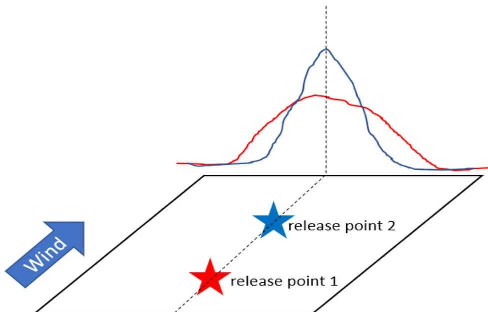
**In this case any release location along the dotted line will result in the same modelled plume-centre location. But a source at release point 2 with a low emission rate will produce the same plume amplitude as a source at release point 1 with a high emission rate. These would produce the same value of J for this transect.**
