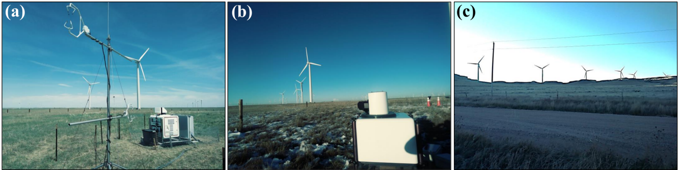
Figure 2. Photos of the LiDAR experiment: (a) LiDAR Windcube 200S and sonic anemometers Campbell Scientific CSAT3; (b) LiDAR Streamline XR; (c) GE 1.5sle turbines of the B row.
