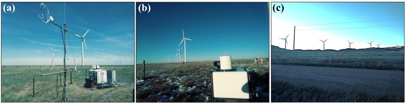
Figure 2. Photos of the LiDAR experiment: (a) LiDAR Windcube 200S and sonic anemometers Campbell Scientific CSAT3; (b) LiDAR Streamline XR; (c) GE 1.5sle turbines of the B row.
