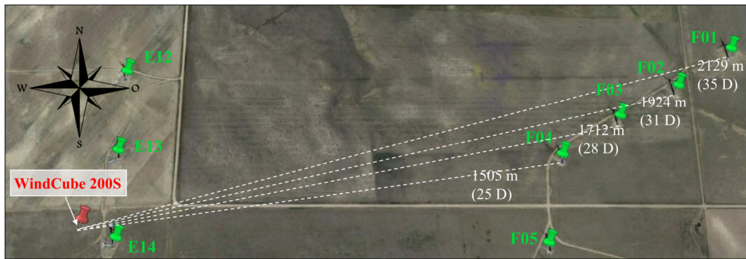
Figure 24. Satellite map of the site for the deployment of the Windcube 200S LiDAR, including the four Mitsubishi wind turbines under investigation. Source: © Google Maps.
