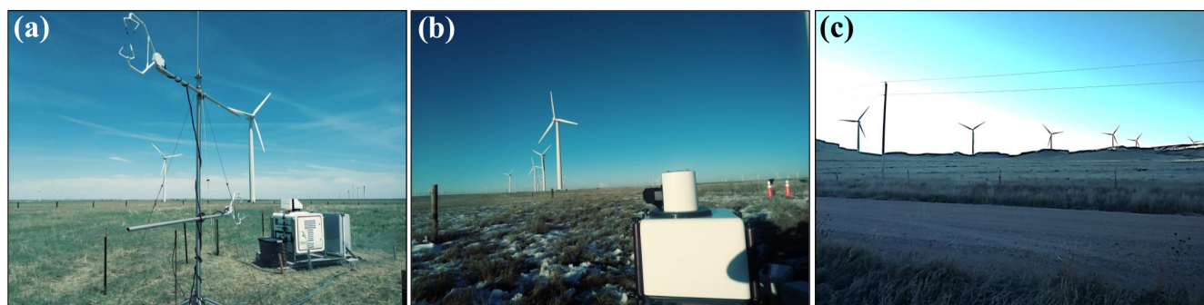
Figure 12. Photos of the LiDAR experiment: (a) LiDAR Windcube 200S and sonic anemometers Campbell Scientific CSAT3; (b) LiDAR Streamline XR; (c) GE 1.5sle turbines of the B row.
