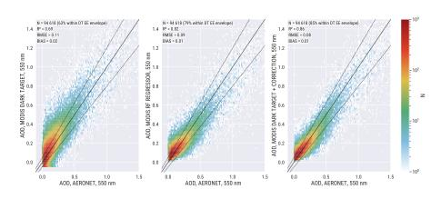
**Figure 3.** Comparison of AERONET and MODIS AOD at 550 nm. Left: MODIS Dark Target over land. Middle: MODIS fully learned Random Forest (RF) based regression model. Right: MODIS Dark Target with RF regression based model enforced post-process correction. The solid black line indicates the 1:1 line. The dashed black lines show the MODIS Dark Target expected error (EE) envelope.
