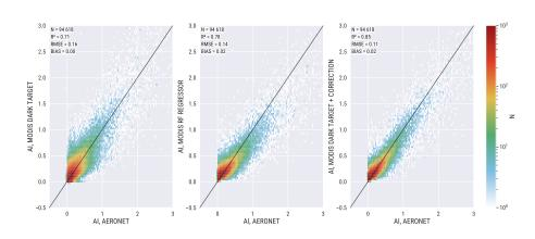
**Figure 5.** Comparison of AERONET and MODIS aerosol index (AI). Left: MODIS Dark Target over land. Middle: MODIS fully learned Random Forest (RF) based regression model. Right: MODIS Dark Target with RF regression based model enforced post-process correction. The solid black line indicates the 1:1 line.
