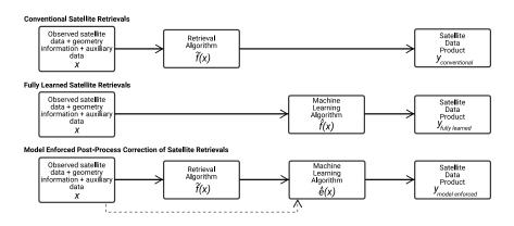
**Figure 1.** Top: Conventional satellite retrieval. Middle: Fully learned machine learning based satellite retrieval approach. Bottom: Model enforced post-process correction satellite retrieval approach.
