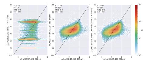
**Figure 4.** Comparison of AERONET and MODIS Angstrom exponent (AE). Left: MODIS Dark Target over land AE 440–660 nm. Middle: MODIS fully learned Random Forest (RF) based regression model AE 440–870 nm. Right: MODIS Dark Target AE 440–660 nm with RF regression based model enforced post-process correction. The solid black line indicates the 1:1 line.
